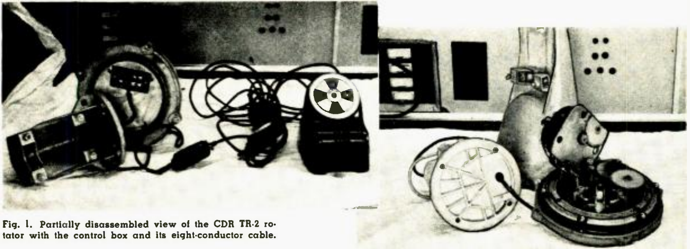
Fig. 2. The motor of the CDR rotator has been swung back to expose the gears. Note the ball bearings around the base.
