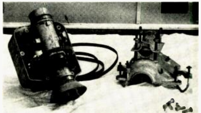
Fig. 5. View of an Alliance rotator showing the worm-gear drive. The dark collar below the main driving gear contains position indicating pot. similar to that shown in Fig. 3.
