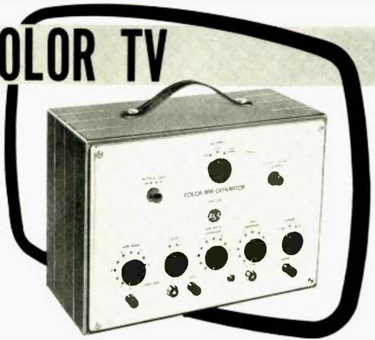
Fig. 1. A color-bar generator is probably the handiest color test instrument. A typical one is the RCA generator shown here.
