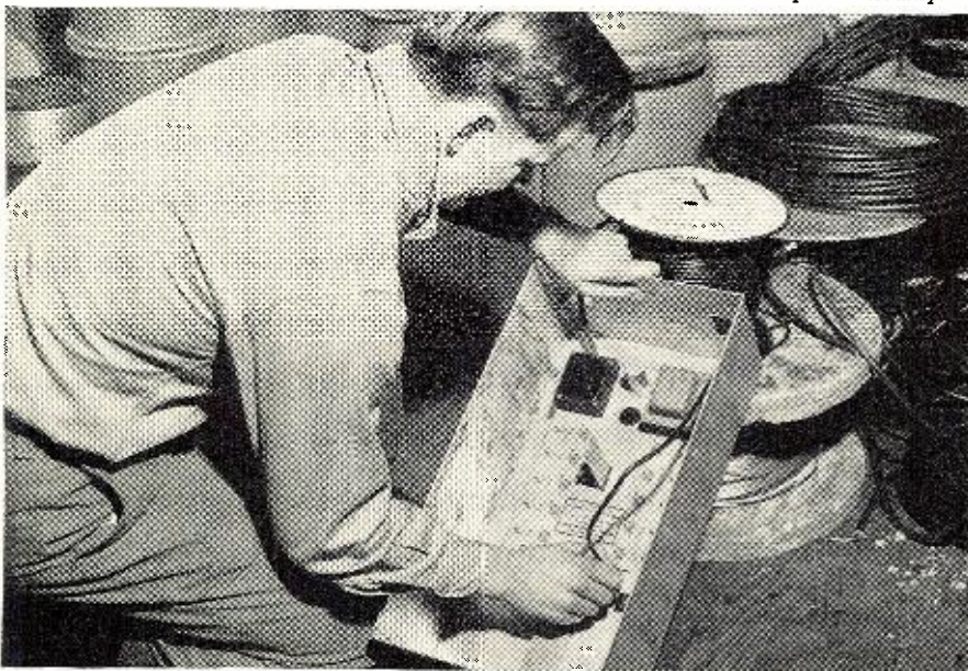
Fig. 8. Wiring an ADO-10 antenna distribution box for use in the Panther Valley "community aerial" system. Signals from Philadelphia's three television stations, seventy airline miles away, are being received in Lansford, Pa., clearly and cleanly.
