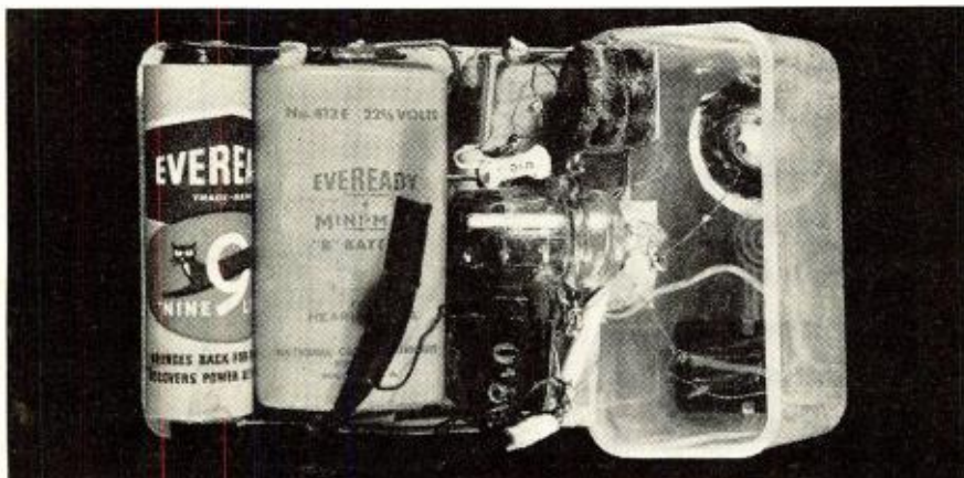
View of vest pocket receiver showing how components are assembled for compactness.
