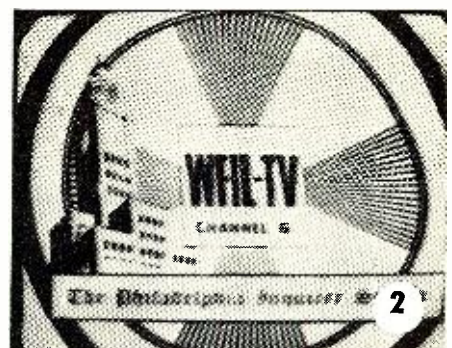
Fig. 2. Slight horizontal pulling, as evidenced by bending of the left and right hand sides of the box around "WFIL-TV," caused by an undesired magnetic field near the picture tube. The pulling, which is present on the raster with or without the picture, may be horizontal, vertical, or both depending on the location of the field. If the field is due to a magnetized portion of the shell of a metal-type picture tube, it may be detected by turning the tube, thus shifting direction of pulling.
