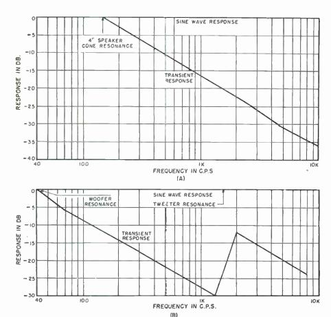
Graph of relationships between sine wave and transient characteristics in ( $\tilde{A}$ ) a hypothetical woofer-tweeter combination, and (B) system using group of identical small speakers.
