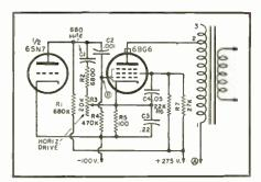
Fig. 5. Diagram of synchrolock drive circuit.
