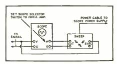
Fig. 4. Method for hooking up sweep unit.
