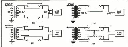
Fig. 9. Functional diagrams of the double jack system referred to in the text.
