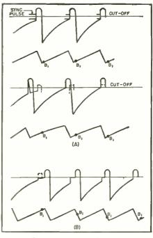
Fig. 3. Effect of noise on blocking oscillator, large pulse tripping oscillator too soon (A), cancelling pulse causing "miss" (B).
