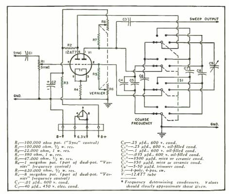
Fig. 3. Complete schematic diagram of the wide-range, multivibrator sweep circult.
