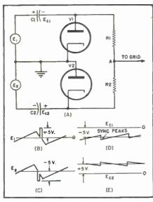
Fig. 5. A simplified schematic diagram of comparison circuit (A) showing voltage  $E_1$  (B), and  $E_2$  (C), and the voltage across the condenser  $C_1$  (D), and across  $C_2$  (E).
