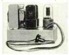
a 75% aural improvement is obtained. according to the distributor. With a quality speaker, the amplifier delivers its full range of 100 to 13,000 c.p.s.
