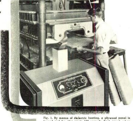
formed and the glue set in 120 seconds. Each panel, when sawed, will yield four curved fronts for radio cabinets.
