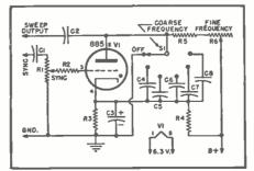
tions, it is often desirable to observe signals as high as several hundred kilocycles, or more. A 30 kc. sweep would present too many cycles of a high frequency signal on the cathoderay screen, and thus make close observation and analysis difficult. For this reason, many of the modern scopes as well as the more expensive units, employ a multivibrator type of sweep, permitting sweeps as high as 100 kc. or more.
