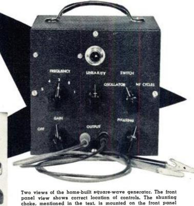
just above oscillator transformer and is visible in the side view. If enclosed cabinet is used vent holes must be provided.
