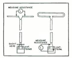
Fig. 3. Checking for bad antenna connections.
