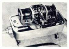
The motor can be remotely controlled in much the same way as a servomechanism. The unit can be used as an antenna rotator, for operating radio tuning and direction finding controls, for operating remote controlled rheostats, etc.
