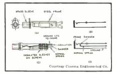
Fig. 10. Construction of standard jacks of the types widely used in sound studios.
