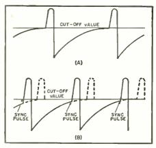
Fig. 2. Blocking oscillator grid voltage, without sync pulses (A) and with pulses (B).
