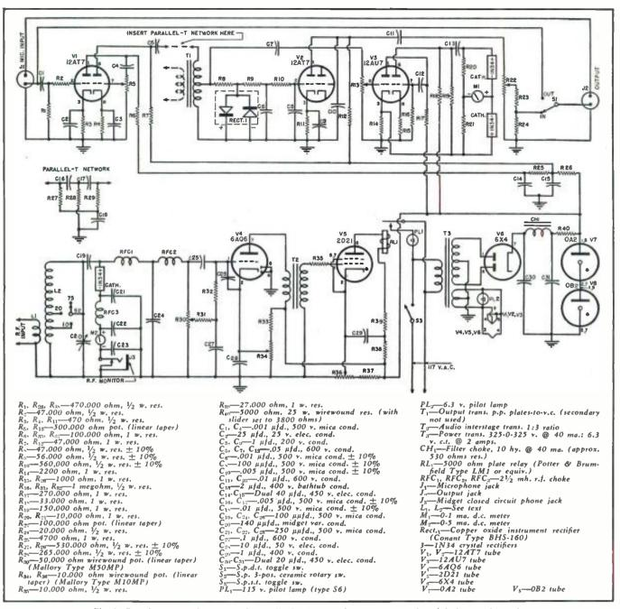
Fig. 4. Complete circuit diagram and parts list for the speech compressor and modulation monitor unit.
