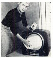
scratch-free, and conditioned against many of the future scratching hazards. Investigation has shown that almost 90% of the scratching of such screens is due to the tiny dust particles, which are attracted to the plastics, being ground into the surface under the pressure of normal cleaning or wiping. These particles are negatively charged and cling to a positive staticcharged screen.
