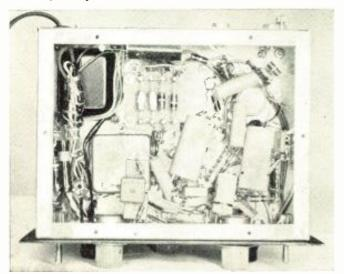
Fig. 7. View of the modulation monitor sub-chassis. Note T<sub>1</sub> behind the r.f. link terminals in "well" of the r.f. sub-chassis.
