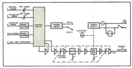
Fig. 2. Block diagram of a preamp-equalizer designed for five input channels.
