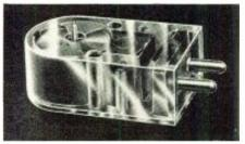
workings of the pickup. The cartridge weighs 14 grams. The compliance is adequate for all types of recordings. The instrument is velocity responsive and is essentially flat, by recording playback standards, to above 10,000 c.p.s. The cartridge is 11/2 inches long.
