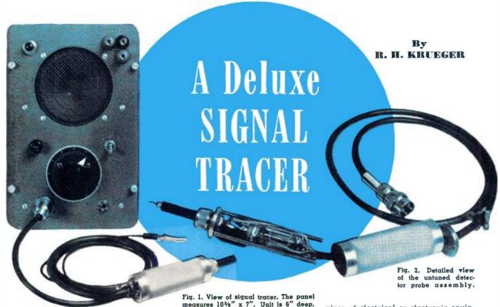
In combining a good, all-purpose, 3-stage audio amplifier and an untuned detector, the author has devised a handy, laboratory-type instrument.
