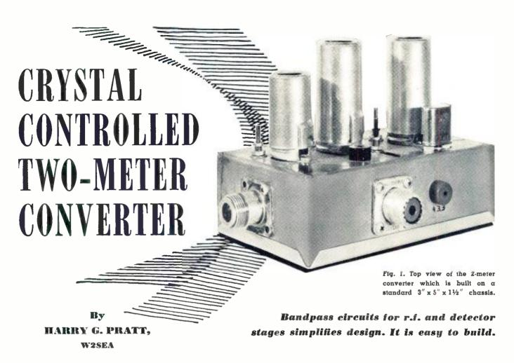
UCH interest has been shown in recent years in improved equipment for the higher frequency amateur bands. Crystal controlled transmitters have been accepted as standard equipment on 2 meters; however, little consideration has been given to increasing receiver stability. The converter described in this article has been designed to provide good sensitivity, stability, and at the same time, ease of operation.
