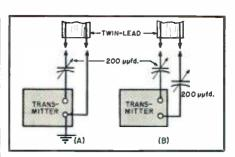
Fig. 3. Methods for feeding the antenna. (A) Unbalanced and (B) balanced methods.
