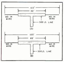
Fig. 2. (A) Mechanical details of 20-75 meter antenna and (B) the 40-75/80 meter antenna.
