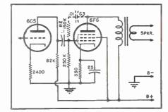
tubes used today have relatively high plate impedance. The use of sufficient feedback can effectively lower the plate impedance, as seen from the loudspeaker end, and increase the damping to a marked degree.
