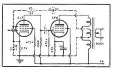
Fig. 5. Instead of obtaining feedback voltage from the voice coil winding as in Fig. 4. a special winding known as a tertiary feedback winding is used. Transformers in corporating these windings are gradually disappearing from the market as less costly methods are used to get degeneration.
