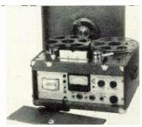
range of 15,000 cycles on half-track tape recorded at 71/2" per second tape speed.
