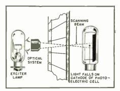
Fig. 2. Mechanical details of input stage.
