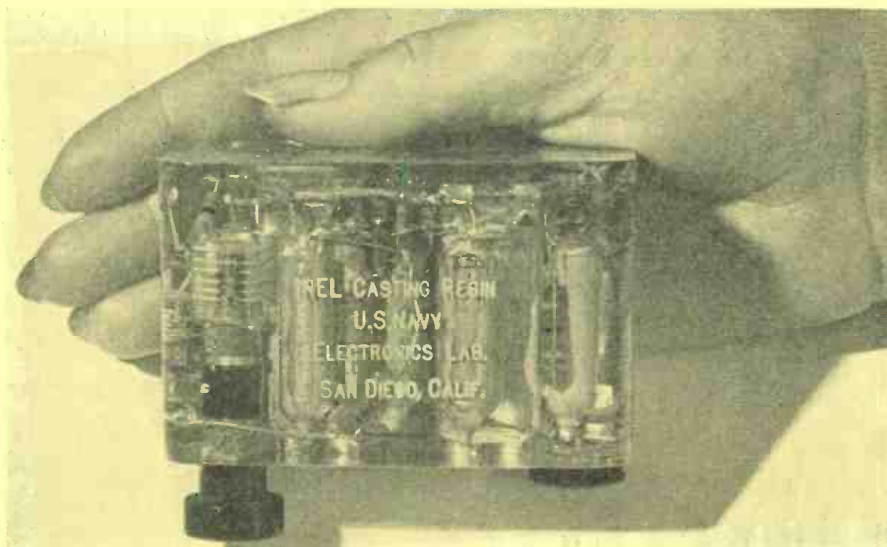
Top view of a complete receiver encased in NEL casting resin.
