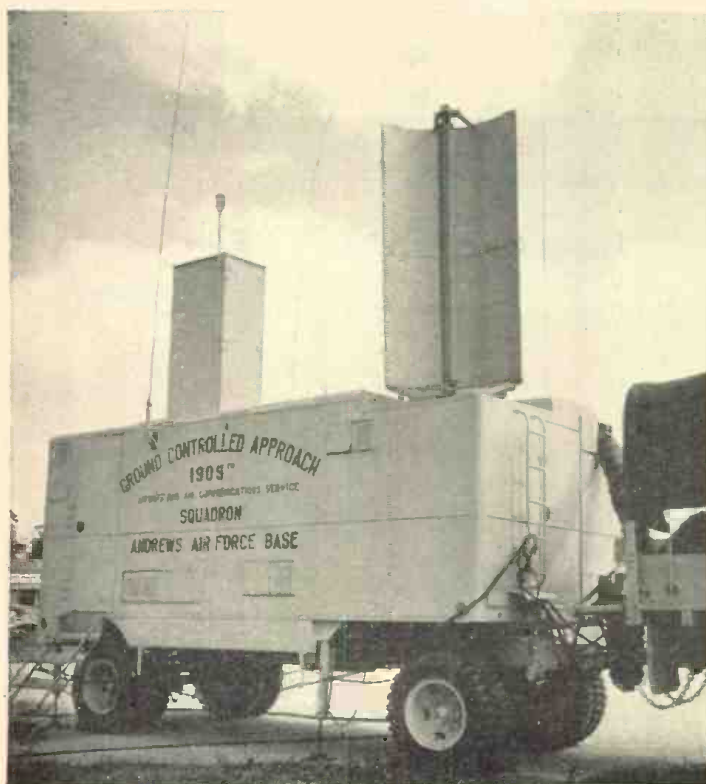
Exterior view of the Ground Controlled Approach equipment.
