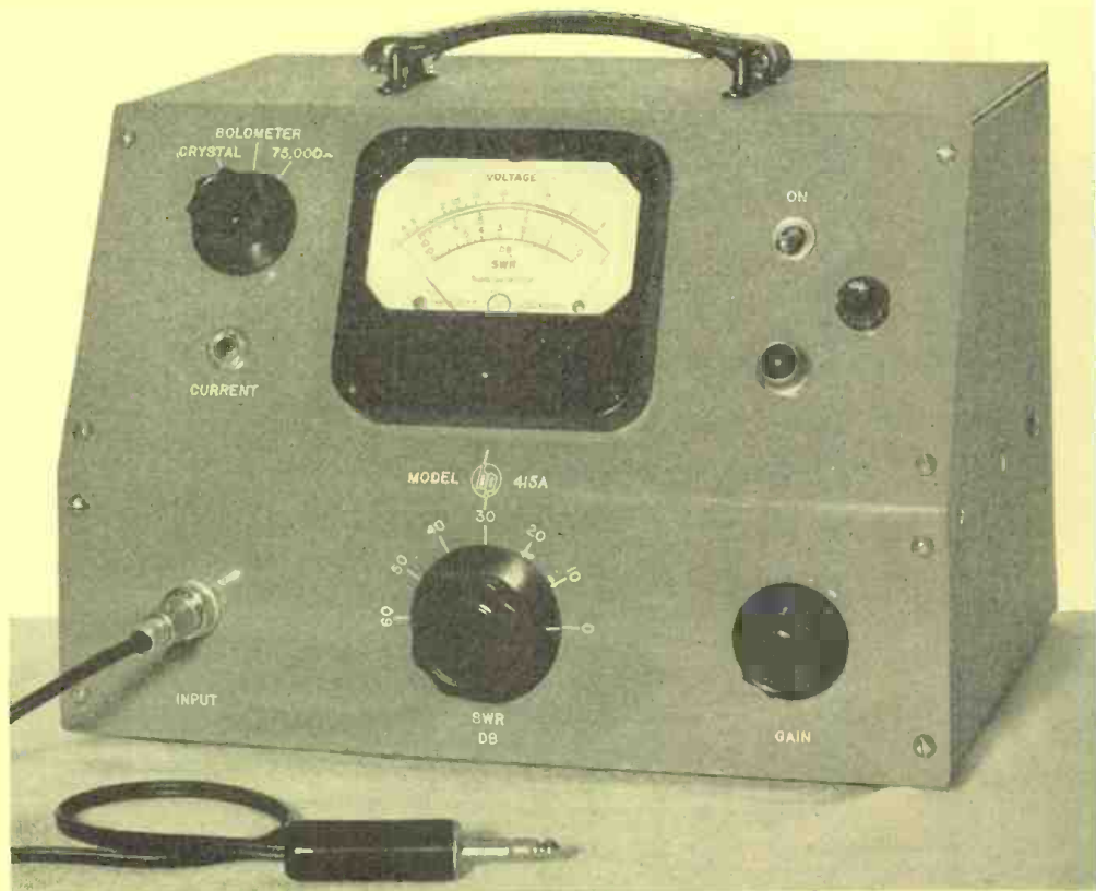
Power meter for measuring standard wave ratios on slotted line. The r.f. is modulated at 1000 cycles and is detected, amplified, and measured by this instrument.
