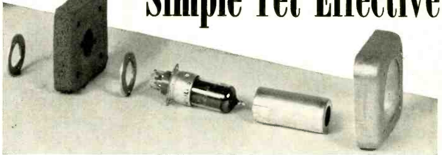
Fig. 1. An "exploded" view of the shock mounting assembly.
