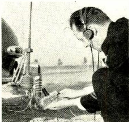
Fig. 7. (Left) Taking a reading of the resonant frequency of the mobile antenna with the "Bloopers." When the audio tone stops in the headphones the resonant frequency is indicated on the dial. The rods used to strengthen the base mounting are also visible. (Below) The antenna is attached to the rear bumper of the car and coupled to the transmitter through a low impedance line.
