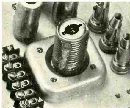
Fig. 4. Top view of shock mounted tube shown in position on equipment chassis.
