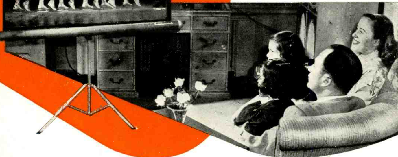
Fig. 1. An adaptation, by Ansley Radio Co., of the Protelgram system which produces a 1728 sq. inch picture.
