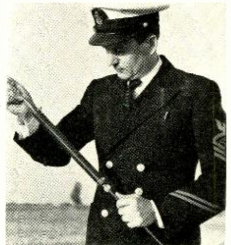
Fig. 5. A close-up view of the loading inductance as used in the mobile antenna.
