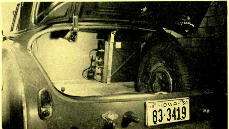
Compactness, making for space conservation, features the transmitter-receiver installation in the manager's car.
