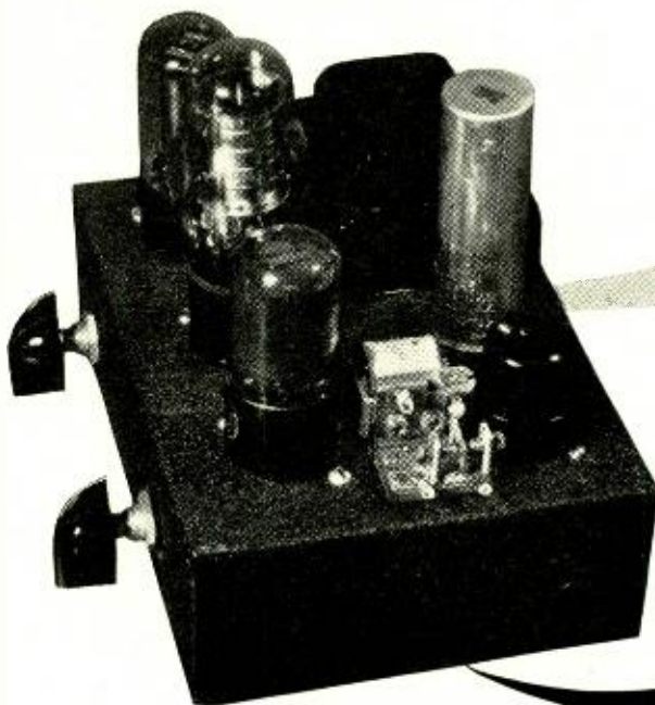
A compact, a.c. operated Wheatstone bridge used as an electronic lock and if desired, for remote control applications.
