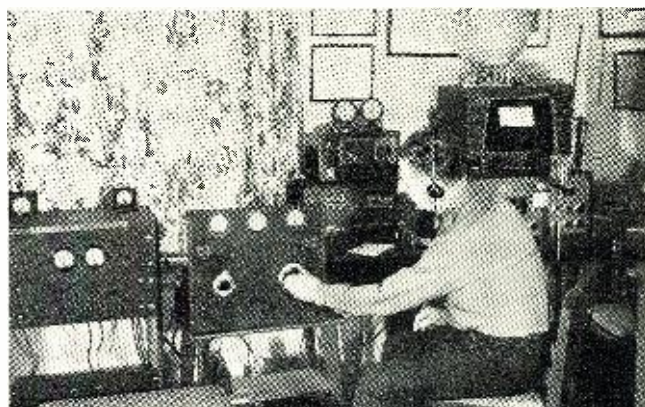
The "ham shack" at W3DF. An HT-18 unit drives either a 600 w. phone or 400 w. c.w. rig. Transmitting gear is home-constructed.
