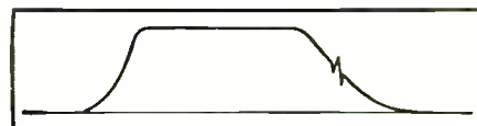
Fig. 4. A video i.f. response curve showing position of marker pip at the point where the video carrier should appear.
