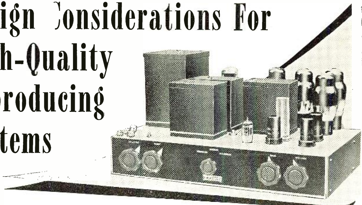
Fig. 1. Over-all view of audio amplifier built by the author. The unit incorporates many of the design features covered in text. Schematic diagram appears on page 72.
