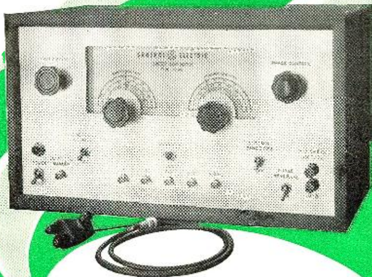
Fig. 1. Front view of the generator. The vernier r.f. output attenuator is at left of the coaxial cable.
