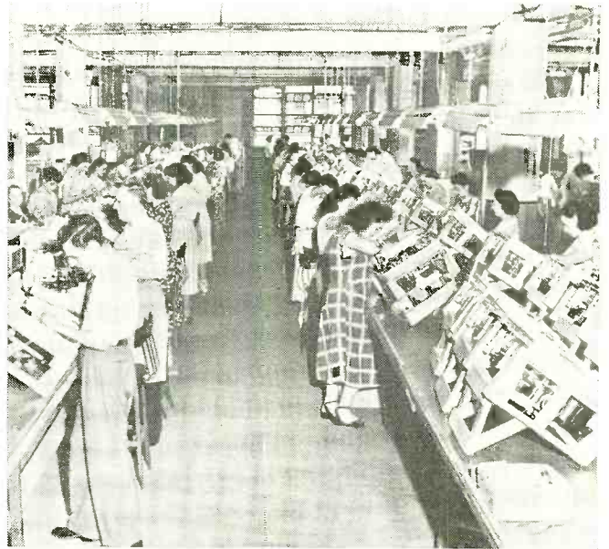
The television assembly line at the Andrea plant. Here table model video receivers are being produced in quantity.
