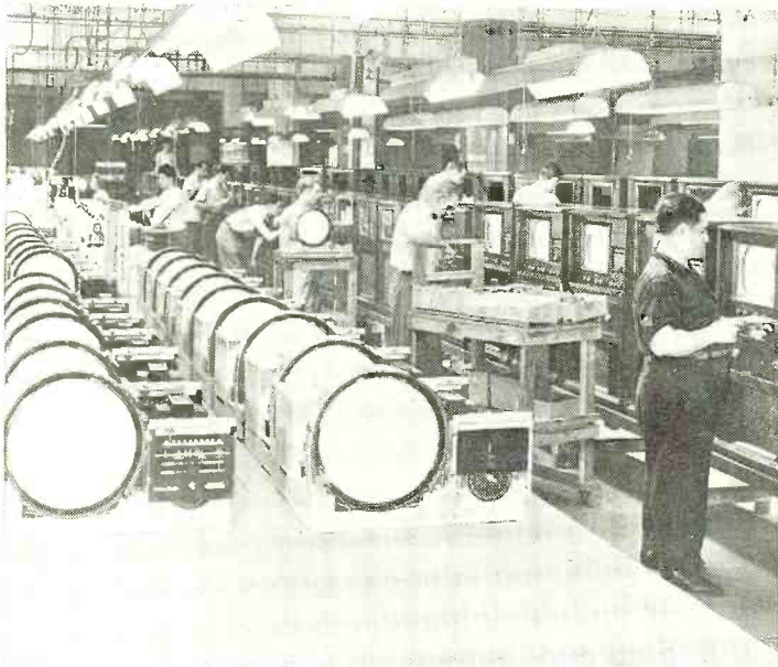
The present-day Andrea cabinet assembly line where the completed chassis are installed into the television cabinets.
