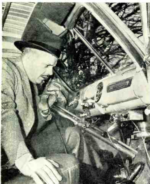
Fig. 4. The mobile unit used in this carrier system is operated through the control head mounted on the instrument panel of the car's or truck's dashboard. Push-to-talk operation is customary.
