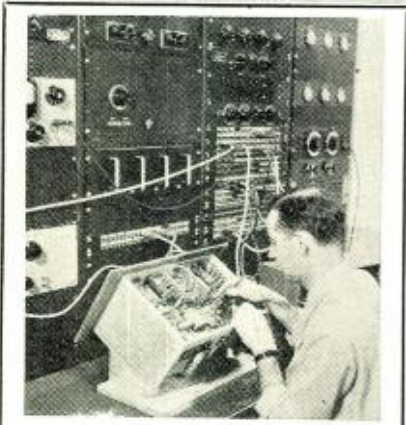
COVER PHOTO: The testing of precision audio equipment requires the use of laboratory instruments to insure proper operation. Here Ernest Baumeister tests an audio filter in the laboratories of Cinema Engineering Co., Burbank, Calif. Further details are given on Page 70. (Photo by Arthur Haug)
