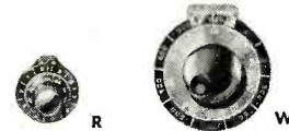
MODELS R AND W DUODIALS Each model available in standard turns-ratios of 10, 15, 25 and 40 to 1. Inner scale indicates angular position of HELIPOT sliding contact, and outer scale the helical turn on which it is located. Can be driven from knob or shaft end. R—2" diameter, exclusive of index. W—4-3/4" diameter, exclusive of index. Features finger hole in knob to speed rotation. — Ask for Bulletins 104 and 114 —
