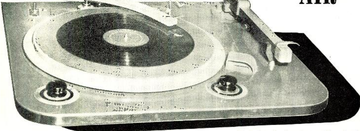
Fig. 1. Typical radio station turntable equipment, adapted for microgrooves. Note conventional pickup arm at right and changeover switch, left rear.
