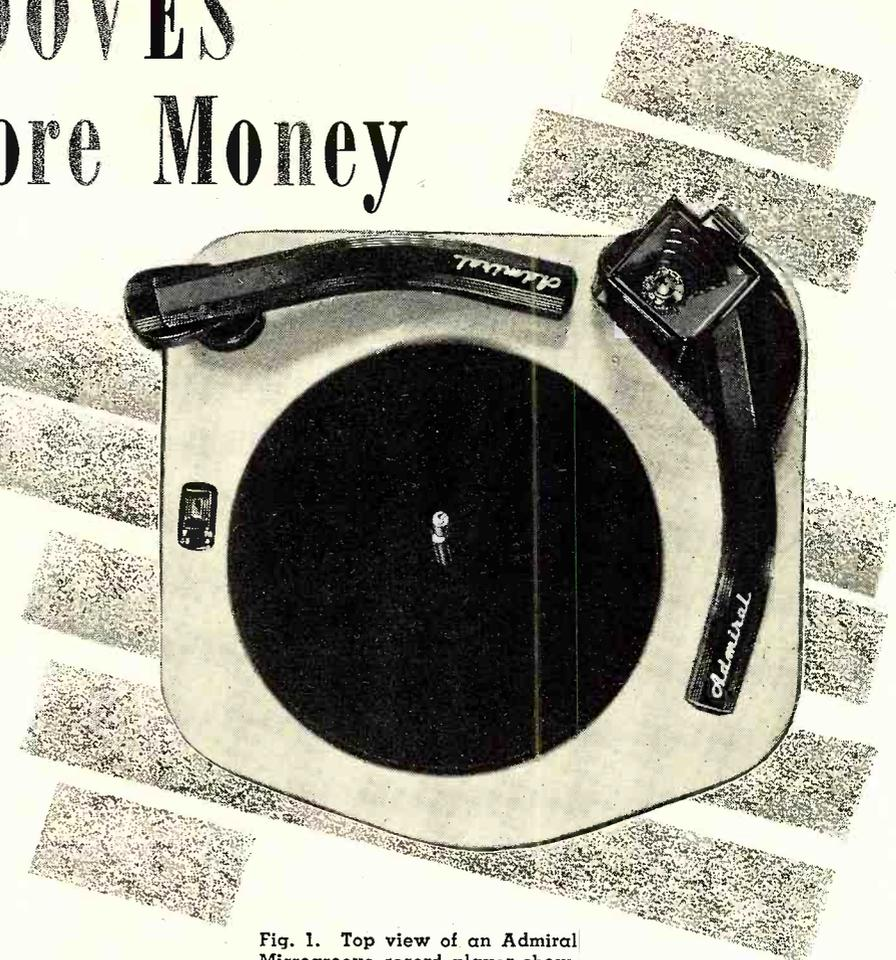
Fig. 1. Top view of an Admiral Microgroove record player showing the two pickup arms used.
