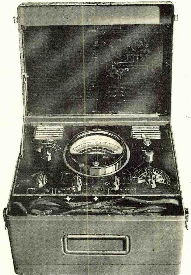
0-60 volts and 0-60 amperes. One switch box indicator has following ranges: 0-9 volts and amperes, scale deviation—0-9 range in 1/10th of a volt, 0-18 in 2/10th's of a volt, 0-60 in 1 volt and ampere division, 0-9 in .05th of a volt and ampere.
