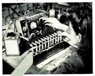
An Aerovox capacitance bridge for measuring capacitance, equivalent series resistance, leakage and other electrical characteristics of electrolytics.
