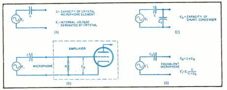
Fig. 6. Step by step analysis of applying a crystal type microphone to pulse wave recording. The standard crystal, as we know it, is not suitable as the time constant RC is too small when used with an amplifier. By adding shunt capacity across this crystal, it can be well adapted to pulse recording equipment.
