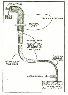
Fig. 6. Example of radar wave guide system.
