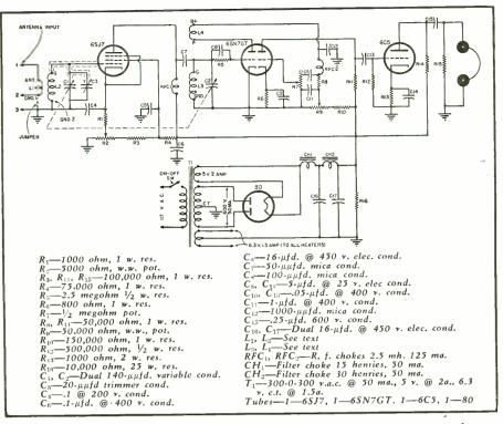
Fig. 1. Diagram of regenerative three-tube short-wave receiver. The power supply is constructed as a separate unit and, if desired, may be replaced by batteries.
