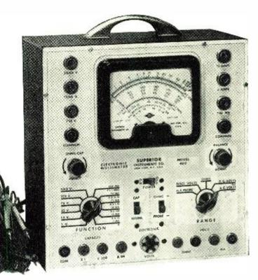
A COMBINATION VACUUM-TUBE VOLTMETER AND VOLT-OHM MILLIAMMETER PLUS CAPACITY INDUCTANCE REACTANCE AND DECIBEL
