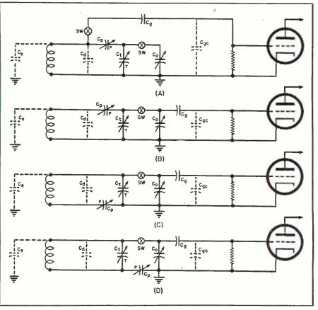
of that employed for grid coil "L." The feedback circuit, shown as a dotted line in Fig. 1 from " $C_p$ ," should also be connected to the ground of the battery " $E_p$ " as this battery also forms a return to produce oscillation.
