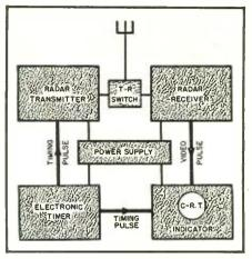
Fig. 13. Single-antenna-radar system.
