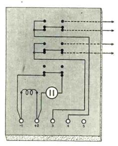
Timer Wiring diagram of time delay relay. must be connected positive and negative as shown, otherwise instrument may be damaged.
