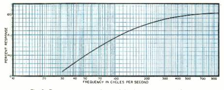
Fig. 2. Frequency response characteristic of the average of a large number of acoustic stethoscopes, minus the effects of the chest piece.
