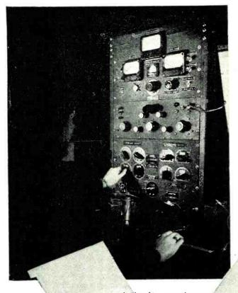
Obtaining the characteristics of aluminum foil samples in order to insure uniform Aerovox quality of each unit throughout production.
