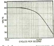
Fig. 2. Frequency response characteristic of a copper-oxide rectifier-type a.c. voltmeter. Its accuracy is undependable over 1000 cycles. It is advisable to employ a v.t.v.m. type meter when making frequency measurements.
