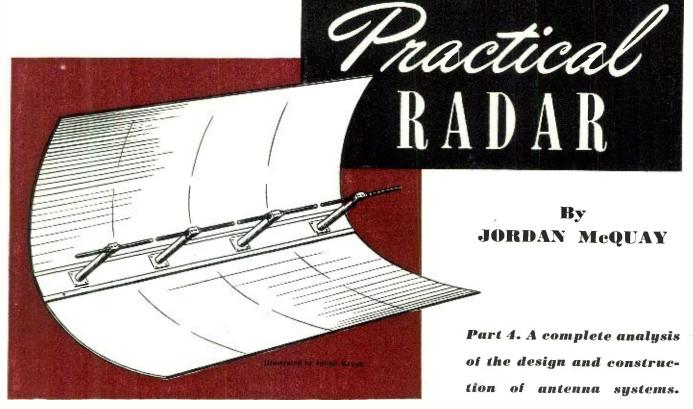
Fig. 1. Antenna used for transmitting u.h.f. pulses.
