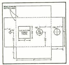
Fig. 3. Power supply chassis layout.
