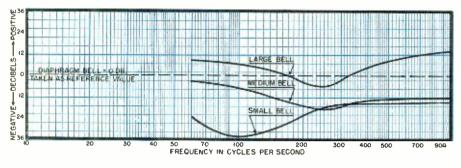
Fig. 3. Resultant curves of the three open chest pieces of Fig. 5, as compared with diaphragm type chest piece. The higher the decibel reading, the higher is the relative efficiency of the chest piece.
