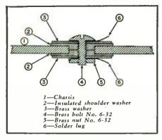
Fig. 2. A novel by pass condensor. It can be cut into the chassis at any desired position permitting short connections.
