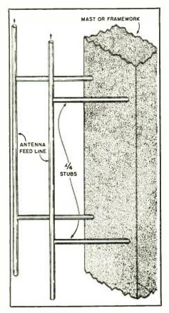
Fig. 3. Use of stub supports.
