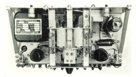
Top view of field detector unit. This instrument has particular application in measuring the radio field strength of airport glide paths.
