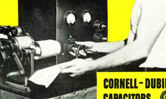
Testing paper for number of conducting particles. Other tests determine thickness, porosity, voltage breakdown.
