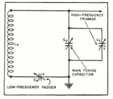
Fig. 1. Basic "padded" oscillator tuning circuit. Low-frequency padding capacitor  $C_p$  is inserted in series with resonant circuit. The oscillator tuning characteristic that will result is shown in Fig. 2.
