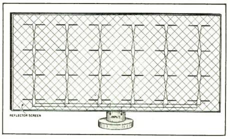
Fig. 9. An ordinary antenna array of stacked dipoles mounted in multiples of four.
