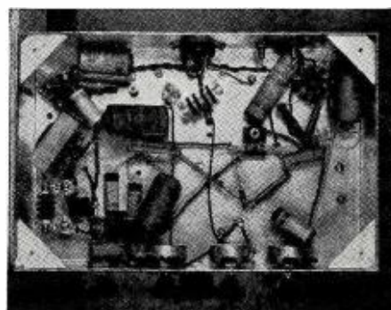
Underchassis view of the T.R.F. unit.
