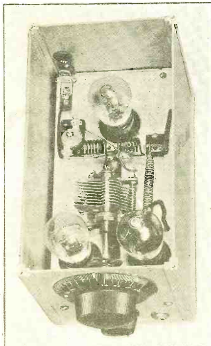
ULTRA SHORT-WAVE RECEIVER Figure 9. A view of a five-meter receiving set with the top shield removed to show simple layout
