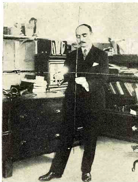
Figure 8. The author holding at right angles two similarly constructed bipoles. Each bipole has at the center of its length a small lamp which lights when current flows in the circuit. Notice that the lamp in the horizontal bipole is glowing, while the lamp in the vertical bipole does not glow. This is because the transmitter on the laboratory table is sending out horizontally polarized waves which cannot be picked up nearby with a vertical antenna
