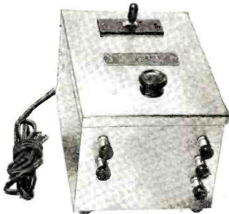
All shielding is plated and highly polished, giving to this receiver a highly attractive appearance
