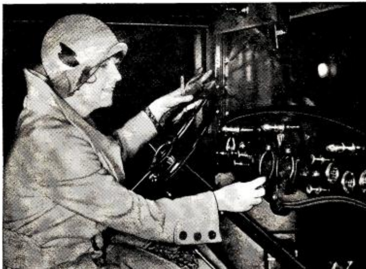
Early Heinafone automobile set in the days before single control was demanded. Installation included a redesigned instrument board to accommodate the radio apparatus
