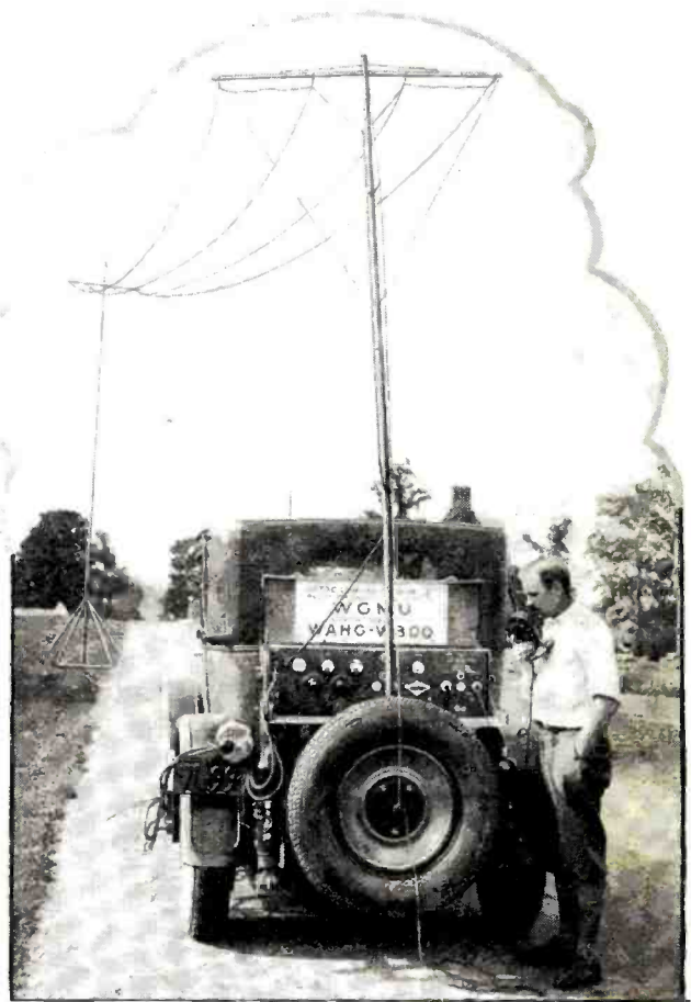
A mobile broadcast transmitter. Such outfits are used to test proposed locations for broadcast stations
