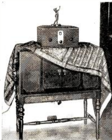
Mounted above the standard broadcast receiver, a simple switch connects either receiver to the loudspeaker
