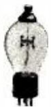
The Piezo—Electric Crystal Mounted in vacuo, with standard 4-prong U X base. Heart of the Stenode System.
