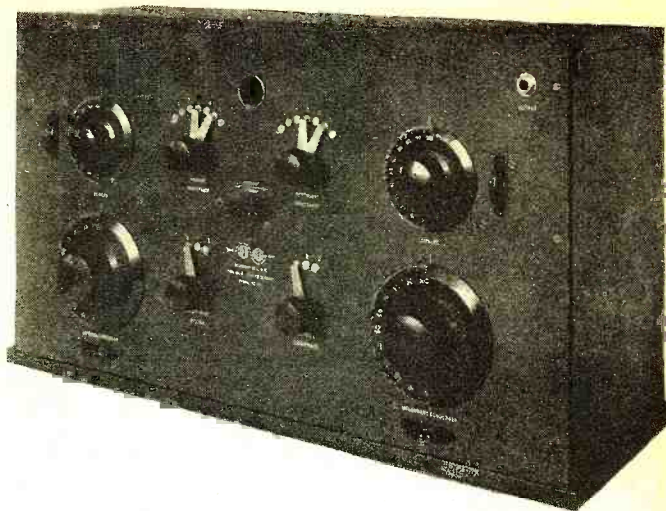
Figure 7. The Grebe CR-7, a high-grade one-tube receiver of 1922, had about everything on the panel but the kitchen sink
