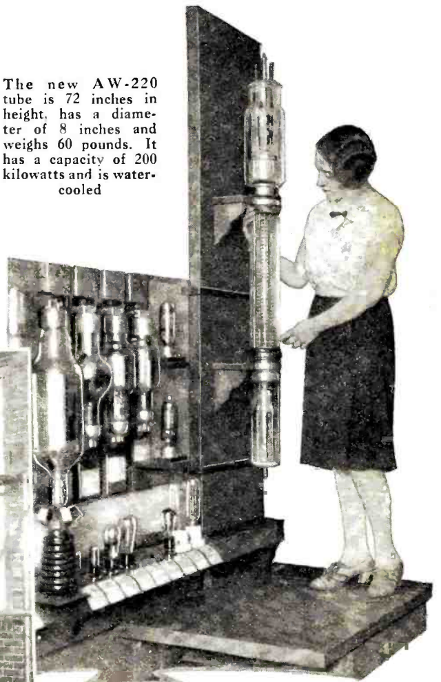
At the left is the power stage equipment of the Saxonburg transmitter and from this panel energy goes directly to the huge spray type antenna designed by Dr. Frank Conrad. Two of the new tubes are shown set up in their tube trucks. The large plates at the right and the coil at the top handle the enormous radio frequency energy generated at this point. They compose the tank condenser of this transmitter and are made of aluminum
