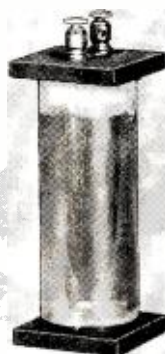
Figure 2. A light sensitive device of the photo-voltaic type, somewhat sluggish in its response to rapid changes in light intensity, but nevertheless finding some commercial uses
