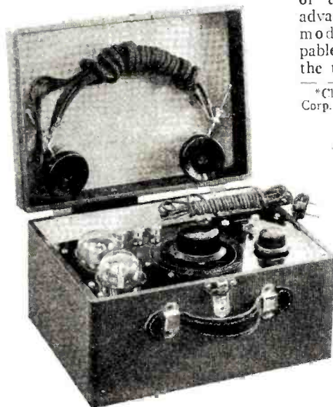
The "Companion" radio open for use. The single tuning control is in the center with the sensitivity control knob at the right
