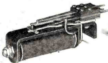
Figure 11. Telephone type relay which is connected into the amplifier plate circuit to provide the necessary link between the phototube equipment and the circuits under control
