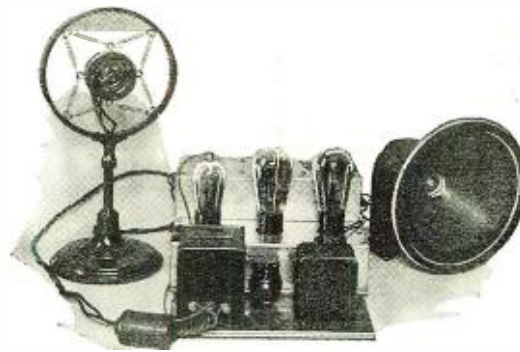
The elements of an easily constructed and amazingly simple "call" system for use in offices. Such an installation is also readily adaptable as a speech amplifier for school, dance hall and similar uses where large outputs of good quality are required. The system comprises a microphone, amplifier and speaker with the attendant coupling transformers and gain control
