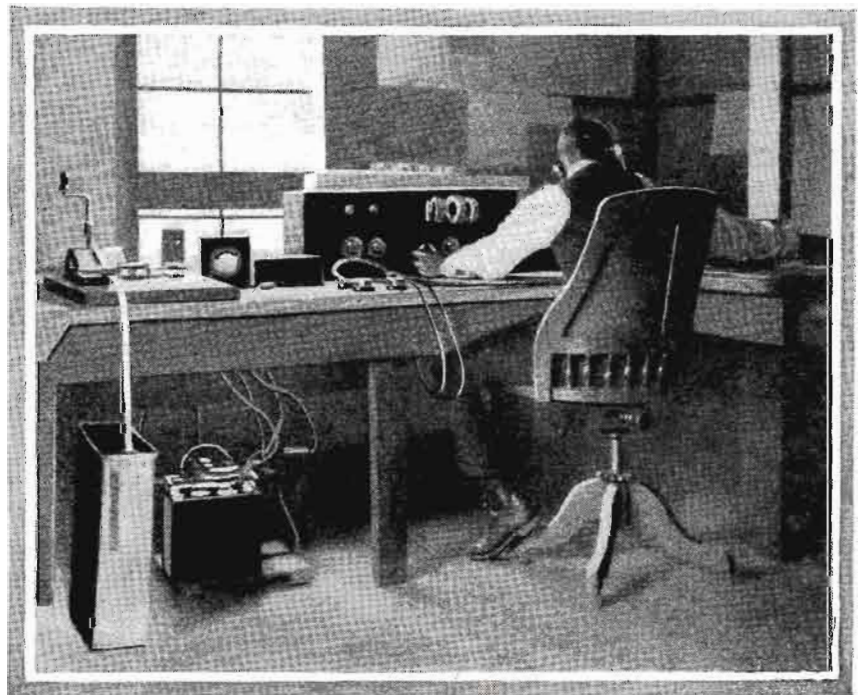
A corner of the static-recording instrument room, showing radio receiver and amplifier.
