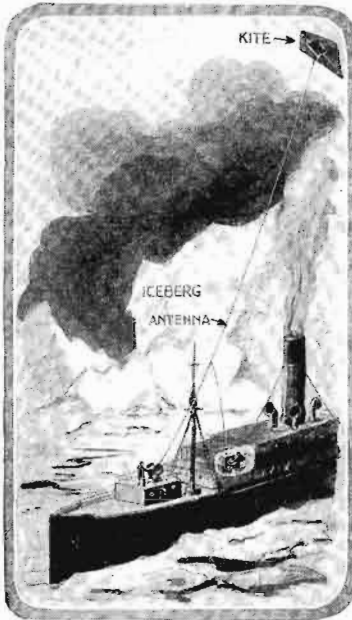
Commander Byrd, who is at the head of the U. S. Navy's polar expedition, expects to use Marconi's original type of antenna for long-distance radio transmission. It consists of a kite, to which is attached the wire that is used as an antenna.
