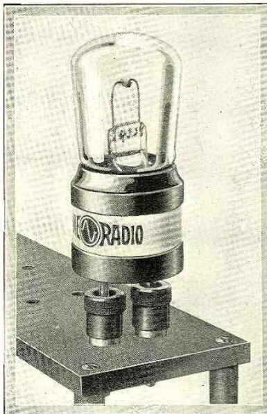
One of the quartz-crystal tubes for the measurement of the frequency of radio-frequency currents.
