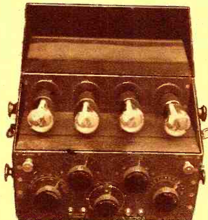
At left, the four-tube regenerative receiver which will be used by the party. It uses French 4-volt tubes, cushioned to absorb shock; 45 and 30 volts "B"; and has one R.F. stage, detector and two of audio.
