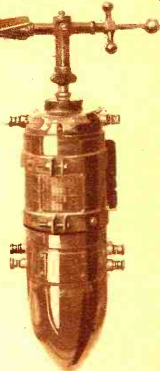
This is a close-up of the generator, and propeller which drives it, to furnish current for the main transmitting set. The single blade is used for better regulation of the speed, which must not vary with that of the plane.
