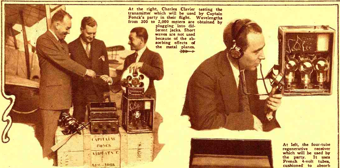
Above, Captain Fonck (right) holding the antenna reel of the French transmitter which will be used; Dr. M. Lionel Stein (center) and Lieut. Snody (left). Beside the latter is the air-driven propeller and generator which gives power for the transmitter.
