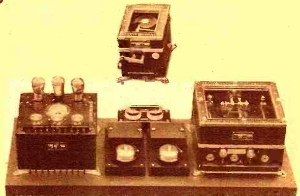
The apparatus shown above was designed to eliminate the constant human watch for SOS signals and will respond automatically to a series of four-second dashes which, it is suggested should be used as a forerunner of all SOS calls. Above is the four-second sender, which is connected to the transmitter; at the left is the receiver and at the right the selector unit for interpreting the signals and ringing the bells in the center. © Herbert Photos.
