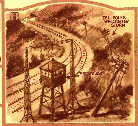
The Milwaukee railroad system has installed a net of short-wave radio transmitters and receivers, over its lines between Chicago and Seattle, which will be especially important in emergencies.
