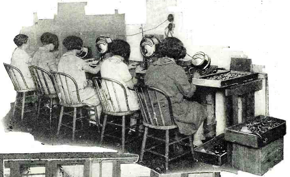
Above is a view of the department in which the resistance strips are first tested. Much care must be exercised at this point, as the impregnated strip is the heart of the apparatus. At the left is the section where the rheostats and potentiometers are assembled.
