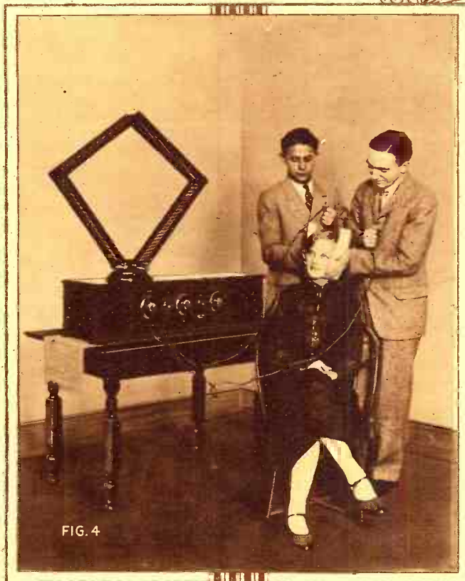
Fig. 4. Here we have a variation of the experiment shown under Fig. 3. Perhaps you do not believe that two sheets of letterhead paper may become a good radio head-set, but hearing is believing, and if you don't believe it, try it and you will have the surprise of your life. Here we have the two performers grasping the two wires coming from the radio set, while their bare hands rest against two letterheads pressed tightly against the young lady's ears. Evidently she is enjoying it, because the sounds are coming through loud and clear with no distortion, and fully as well as with a good head-set. The principle, by the way, is that of Dolbear's Condenser Telephone. Fig. 4A indicates the connections.
