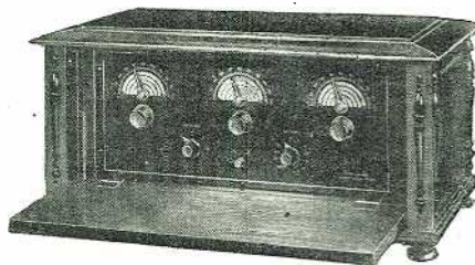
Exterior view of the Renaissance Model, Grimes Inverse Duplex Receiver, incorporating the 4-DL circuit described in these columns.
