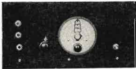
Front view of single control receiver, showing vernier dial used for tuning.
