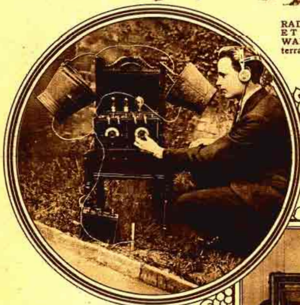
TIN BUCKETS USED AS ANTENNA. This Englishman of Sheffield uses two buckets for an antenna to pick up London and Manchester. He reports excellent reception with this unique receiver. © Underwood & Underwood.
