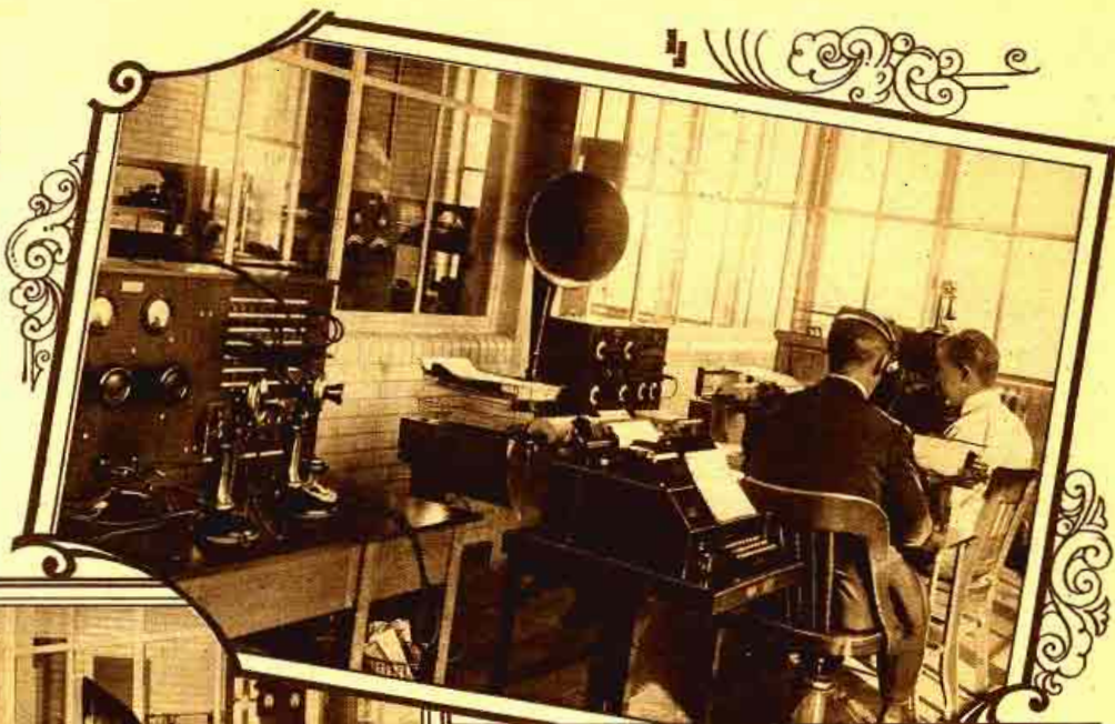
FORD USES RADIO FOR INTERPLANT COMMUNICATION. Two interior views of the radio station at Henry Ford's plant at Dearborn, Mich. In each of the stations are electric typewriters which transmit messages to reproducing typewriters in the various departments. © United.
