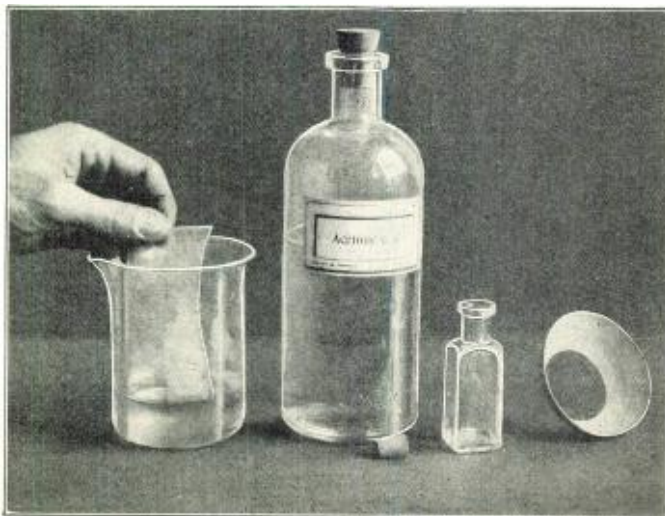
Dissolving the Cleaned Strips of Photo Film in Acetone to Make the Transparent Insulating Varnish. A Formed and Coated Variometer Rotor Can Be Seen at the Right. It is Very Rigid. Simply Flow the Varnish on Your Coils with a Brush and it Will Be Dry in Two Minutes!
