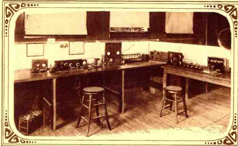
Station 8YAE is Well Laid Out and Lends a Pleasing Appearance to the Eye. The C.W. Set is Only a 10-Watter, But Has a 2-Amp. Kick that Jars Phones on the West Coast. There Are Two Receiving Sets; One a Single Circuit Regenerative, Covering 150 to 400 Meters; and the Other, a B.C. Receiver with Power Amplifier. Note the G.R. Wave-Meter to the Extreme Left of Table.
