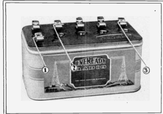
Fig. 4—The new "C" Battery connections for the UX112 tubes. Wire 1 is the minus, 22½ volts for the UX120 tube. Wire 2 the minus, 4½ volts for the first audio tube UV199. Wire 3 the plus "C," common for UV199 and UX120
