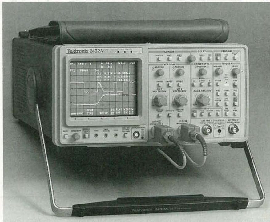
FIG. 7—THE TEKTRONIX 2432A DSO has a 300-MHz bandwidth and a 250-megasample/s digitizing rate. The 2432A includes signal averaging that reduces noise on repetitive signals. A smoothing feature uses a digital low-pass filter to improve the SNR for single-shot waveforms. There's also an AutoStep feature that lets a user build and run test procedures automatically, or by computer via GPIB.
