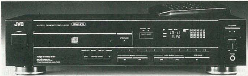
FIG. 11—THE FIRST CD+G/M PLAYER on the market is JVC's XL-G512. It decodes information contained in a CD + G disc's subcodes to output a video signal, and can also output MIDI control information for MIDI-equipped instruments and computers if that information is included on the disc.
