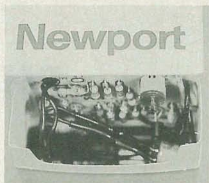
FIG. 6—AN EMPTY CIGARETTE PACK makes a good home for the FM transmitter.
