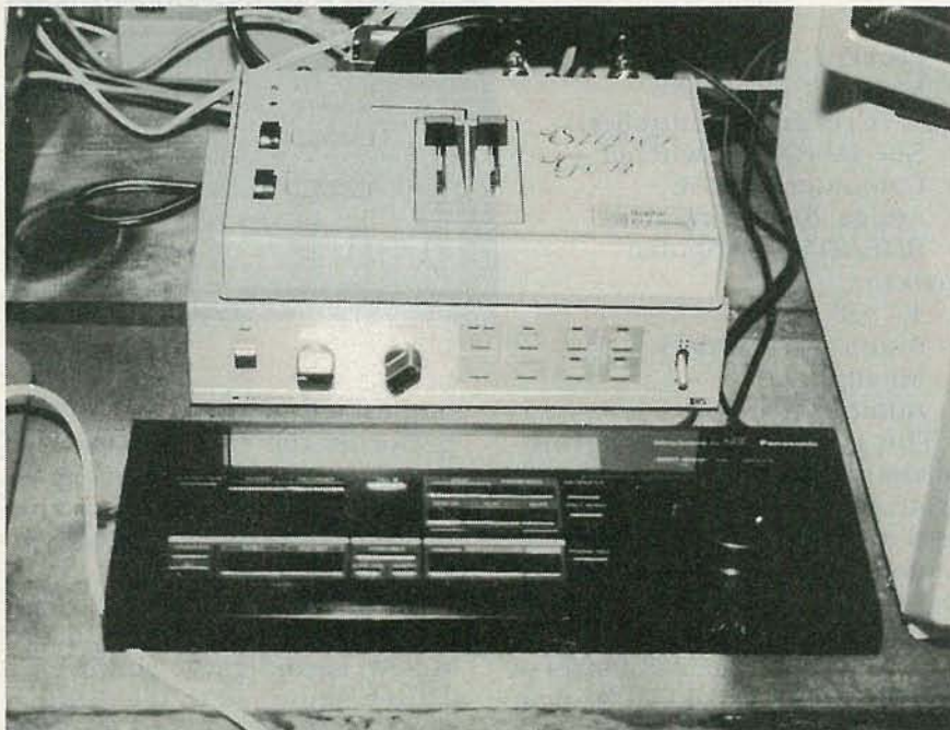
Fig. 2 THE SUPERGEN GENLOCK (top) has manual sliders for graphic fades. The Radio Shack special effects generator (middle) does fades and wipes to black, in addition to switching between two sources. The Panasonic controller (bottom) queues the VCR's for automatic edits.
