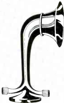
FIG. 9—ONE OF THE EARLIEST ATTEMPTS to get more volume was a small horn that fitted over an earphone.
