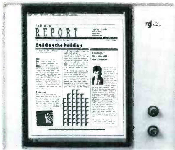
FIG. 4—NEW MONITOR TECHNOLOGIES allow you to see an entire page of text at a time, and make working with CAD and desktop-publishing programs easy. Shown here is the Genius, made by Micro Display Systems.
