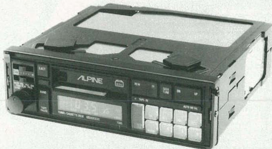
WORRIED ABOUT THEFT? Some receivers, like this one from Alpine, can be slipped out of the dash easily for concealment.
