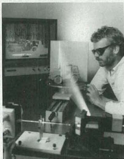
MODEL MAKING. General Electric scientist Daniel Thompson is preparing one of the many images required to make the three-dimensional model from which the jeep could be identified.
