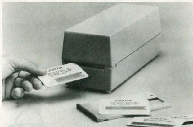
FIG. 6—HOSPITAL ADMISSIONS INFORMATION is contained in a Datastrip on a credit-card size piece of plastic. A special reader reads the data.
