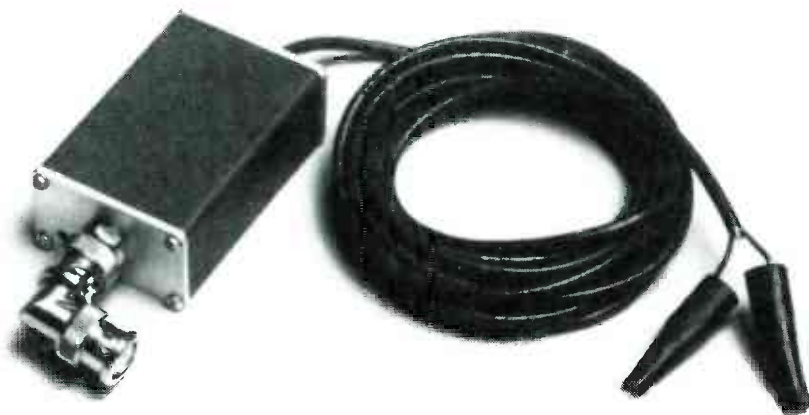
FIG. 8—AN ISOLATION NETWORK is available for the 1503; the network improves noise immunity.
