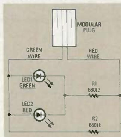
FIG. 18—A SIMPLE TELEPHONE-LINE TESTER. The LED's indicate whether a line or jack is wired correctly, has reversed polarity, or is disconnected from the telephone system.
