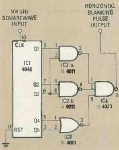
FIG. 4—THE FIRST FIVE COUNTS of a divide-by-32 counter can be used to recreate a horizontal blanking pulse.
