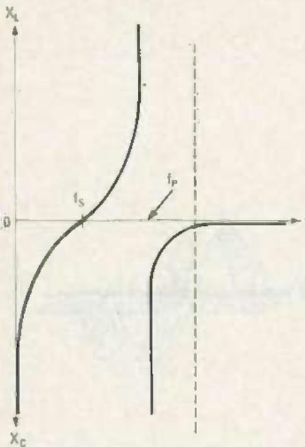
FIG. 3—THE RESONANT FREQUENCY ( $f_s$ ) of a series-mode crystal occurs when the inductive and capacitive reactances are both zero. The resonant frequency ( $f_p$ ) of a parallel-mode crystal occurs when capacitive reactance is zero.
