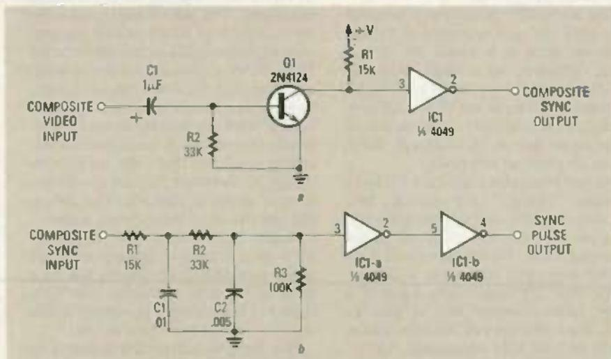
FIG. 3—PART OF THE VIDEO AMPLIFIER'S OUTPUT is picked off and led to a sync separator, which is similar to the ones found in standard TV sets. The output of the separator is used to recover the video sync via a vertical integrator. Typical versions of those two circuits are shown here. The vertical integrator is shown in *a*; the sync separator is shown in *b*.
