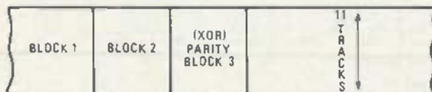
Fig. 2—THE PC/T APPRACH uses a single head to write data to tape in two 4K blocks. Using the same data as in the first two blocks, a third parity block is constructed by performing an exclusive or operation. In this way, should data be lost, it can be more easily reconstructed during an error recovery pass. This does increase system overhead.
