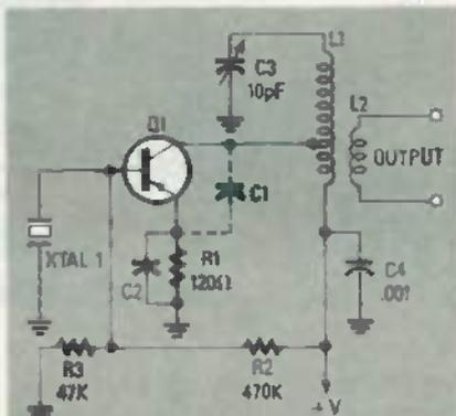
FIG. 7—AN OVERTONE OSCILLATOR also requires few components. As with the Miller oscillator, the L1/C3 circuit should be tuned to a frequency that is near, but not equal to, the frequency of the crystal.
