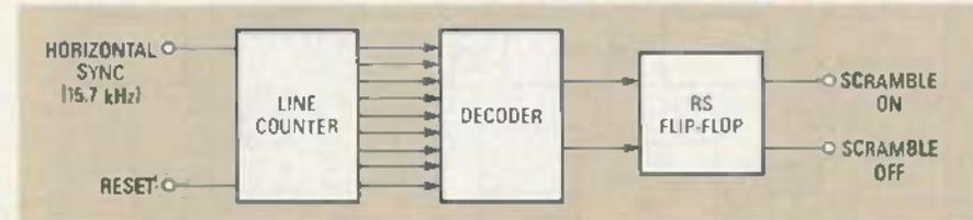
FIG. 6—THE INVERT-LOGIC stage is shown here in block diagram form. That stage controls whether video from the video amp or from the video inverter reaches the output.
