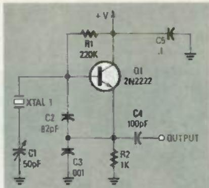
FIG. 6—THE COLPITTS OSCILLATOR comes in various forms; the one shown here is probably more widely used than the one shown in Fig. 4.
