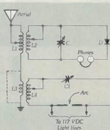
FIG. 9—AN EARLY HETERODYNE RECEIVER. Designed by Fessenden, it used a tuned electric arc as the local oscillator.
