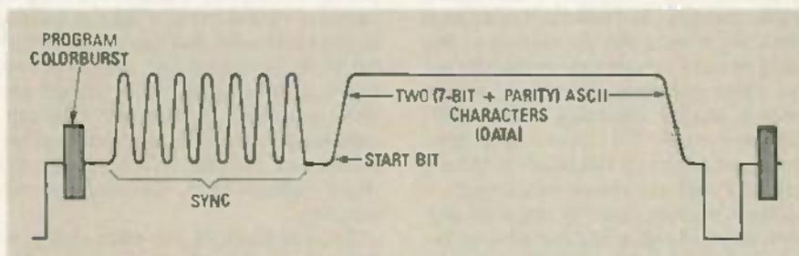
FIG. 1—THE 21ST LINE of each frame of a TV picture contains 17 bits of information. One is a start bit, and two are parity bits. The remaining 14 bits comprise two seven-bit characters of ASCII-like data.
