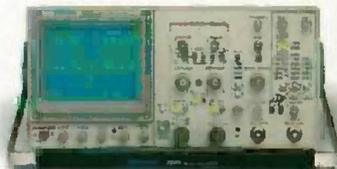
Featuring four channels, flexible triggering, extensive CRT readouts and push-button ease of use, the new Tek 2246 (left) and 2245 (above) bring high-quality, low-cost analysis to diverse applications in digital design, field service and manufacturing.
