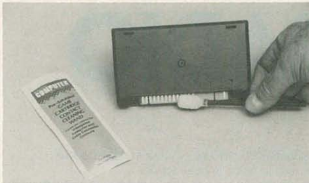
FIG. 8—SOME COMPUTERS and peripherals don't use gold plated edge connectors. If the fingers are simply tinned with solder or even tin plated they can develop intermittent contacts. If you suspect the fingers, just scrub them clean with the same kind of cleaning wand or stick used to clean game cartridges (game cartridges use similar edge connector).
