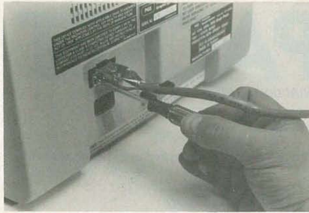
FIG. 10—THE WEIGHT of the relatively heavy shielded hoods commonly used on monitor cables often works them free after several months. Simply tightening the hood's locking screws (if you didn't use them—which is not unusual) is often the cure for an intermittent monitor.
