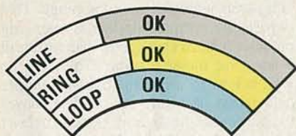
FIG. 5—IF YOU WANT to dress-up the meter, a new scale, similar to the one shown here, can be made. If you choose to do that, be sure that the LINE OK and LOOP OK reference lines fall at the 0.3 mA mark; the RING OK range begins at 0.4 mA.
