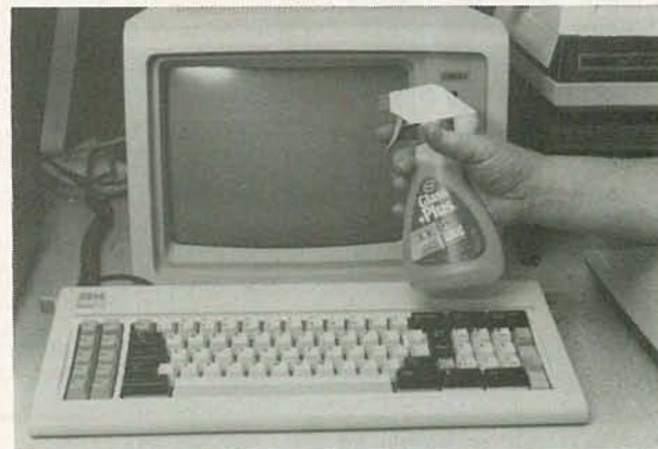
FIG. 2—AN UNSHARP, FUZZY SCREEN display is usually the result of dust on the face of the CRT rather than an electrical breakdown. You can save an expensive "overhaul" service charge if you simply clean the CRT with a common household glass cleaner. (Special CRT cleaning products don't justify their extra cost.)
