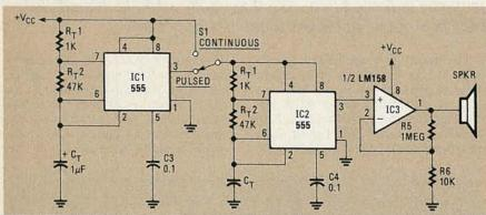
FIG. 3—THIS CIRCUIT IS ideal for experimenting with ultrasonic signals. It can supply either a pulsed or continuous output.
