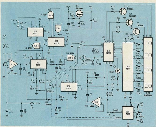
FIG. 2—DWELL/TACHOMETER SCHEMATIC. As shown, the meter is set for 4 cylinders, low tach range. Because the TL092 op-amp that the author used is very hard to find, you might want to substitute National Semiconductor's LM358 for IC1.
