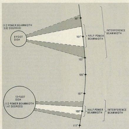
FIG. 4—THE DISH'S SIZE directly affects it beamwidth. As is shown here, the smaller diameter the dish, the larger the beamwidth. That can prove to be a problem for small diameter dishes if two-degree spacing is used. In that case, signals from adjacent satellites can be a source of interference.
