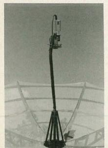
FEED-SUPPORT ARM places the feed and LNA (or LNB/LNC) at the focal point of the dish. The feed arm adjusts in and out to ensure precise setting for maximum signal.
