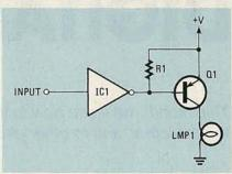
FIG. 8—A MORE COMMON METHOD of interfacing a TTL inverter with a lamp is shown here.
