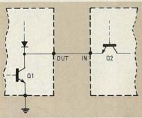
FIG. 1—THE INPUT AND OUTPUT STAGES of a TTL IC are shown here. As is indicated, no special interfacing circuitry is needed when going from the output of one TTL device to the input of another.
