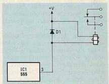
FIG. 12—AN LED, LAMP, OR RELAY (as shown), with a current requirement of less than 200 mA, can be interfaced directly with a 555 timer.
