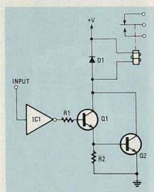
FIG. 11—THE USE OF A DARLINGTON PAIR allows a TTL inverter to control a relay or solenoid with very high current requirements.
