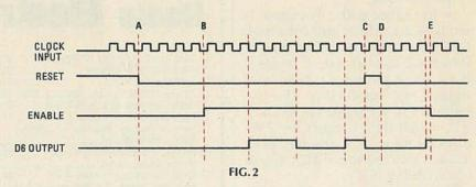
of from +5 to +15 volts. The output is low-power TTL compatible when the IC is operated from a +5-volt supply. The clock input can accept a 50 or 60 Hz sinewave directly thanks to the inclusion of an onboard pulse shaper. The output is in squarewave form, except for the RED 5/6 when used in the divide by 5 mode. Inputs, in addition to the clock input, include 50-/60-Hz division select, input enable, and reset. All of the inputs are protected.
