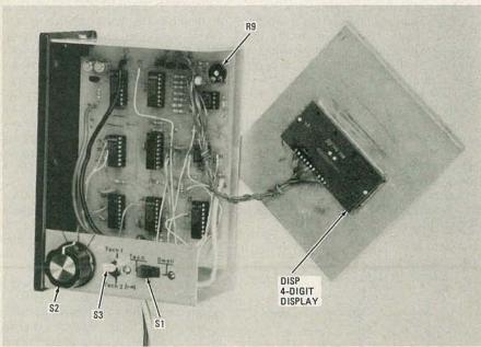
FIG. 3—THE AUTHOR'S PROTOTYPE shown with the cover removed. Note that the display is simply glued to the front panel.
