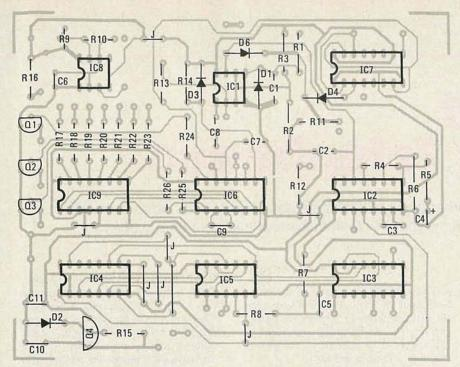
FIG. 4—PARTS PLACEMENT PATTERN for the dwell/tachometer. The PC board pattern is shown in our new "PC Service" department.
