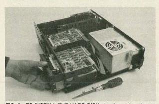
FIG. 2-TO INSTALL THE HARD DISK simply unplug the cables from the floppy B: drive, remove the two screws that secure the drive and slide the floppy drive out of the cabinet, replacing it with the half-height hard disk.
