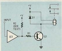
FIG. 10—FOR RELAYS WITH CURRENT requirements that exceed 30–40 mA, this interfacing circuit can be used. Diode D1 is used to keep the level of any inductive spikes to less than 0.7-volt.
