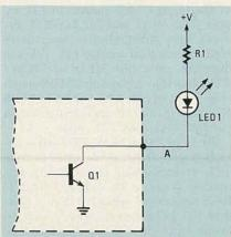
FIG. 6—WHEN THE INPUT TO THE INVERTER is high, the voltage at point A will be close to ground, causing current to flow through the LED, lighting it.
