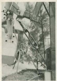
ELEVATION is set on this antenna with turn-buckles.
