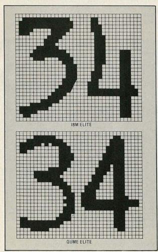
FIG. 4—THE CHARACTER-RECOGNITION ALGORITHMS in an advanced OCR device, such as that made by DEST, is generic. This means it is capable of recognizing a wide variety of typestyles from various manufacturers.
