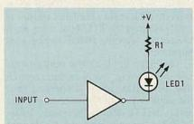
FIG. 5—THIS CIRCUIT SHOWS HOW a TTL inverter can be interfaced to an LED.
