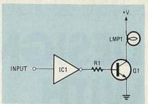
FIG. 7—WHEN THE INVERTER'S OUTPUT is high, the transistor conducts, causing current to flow through the lamp, lighting it.
