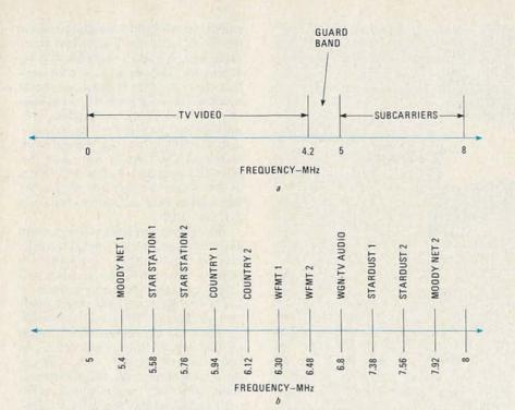
FIG. 3—A TYPICAL TRANSPONDER SIGNAL consists of the video signal, a guard band, and a number of audio subcarriers (see a). The audio subcarriers for F3R, transponder 3 (WGN) is shown in b.
