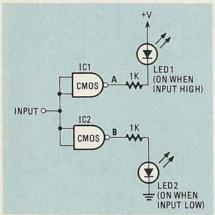
FIG. 4—THIS CIRCUIT SHOWS HOW a CMOS gate, configured as an inverter, can be used to control an LED indicator.
