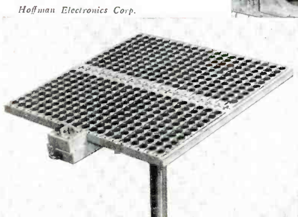
Fig. 4—A 400-cell solar-power converter featuring an automatic sun-following device.
