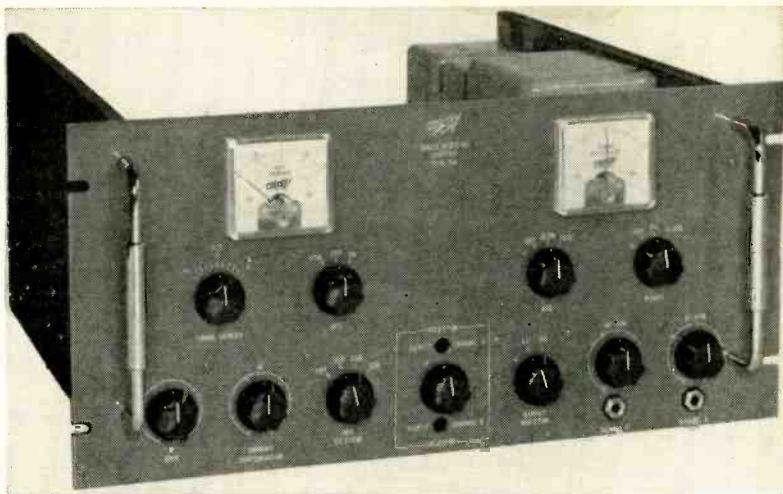
The Crosby type 51A SSB adapter.
