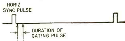
Fig. 4—The color-sync circuits are "open" only for the duration of the burst-amplifier gating pulse.
