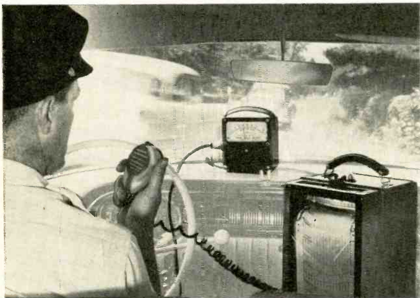
Police officer checks speed of passing cars from his stationary vehicle. Speed meter on top of dash indicates passing vehicle is traveling 40 miles an hour, while recorder at right keeps a permanent record of speed.
