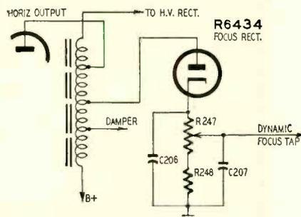
Fig. 7—RCA focus rectifier circuit.
