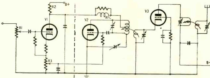
In any high-frequency oscillator (like V2), the frequency increases with a more positive plate voltage or a more negative grid voltage. Either of these changes adds to the grid-plate potential difference, and reduces the transit time between elements. Such voltage variations also affect the amplitude of the oscillations. A more positive plate voltage increases output, while a more negative grid voltage reduces it.
