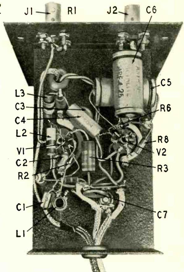
(Fig. 1). For example, if the sweep generator is set at a center frequency of 6.455 mc and mixed with a fixed 6.0-mc signal, the output will consist of the sum and difference of these frequencies as well as the two original signals. However, all the frequencies in the plate circuit of the mixer will be attenuated except the difference frequency, 455 kc. Since the sweep generator is sweeping about 6.455 mc, the output will vary about a center frequency of 455 kc.
