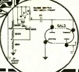
Full wave rectifier in AC input circuit. Read peak-to-peak and RMS volts with upper limit of 4000 P-P and 1500 volts RMS. Voltage divider input circuit.
