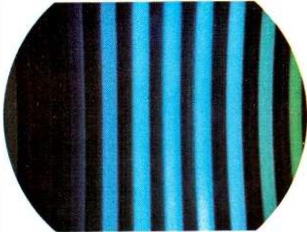
Fig. 7—Color bar pattern with red information missing.
