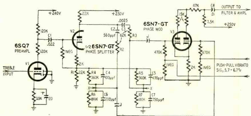
Fig. 4—Schematic of the vibrato circuit—less low-frequency oscillator.
