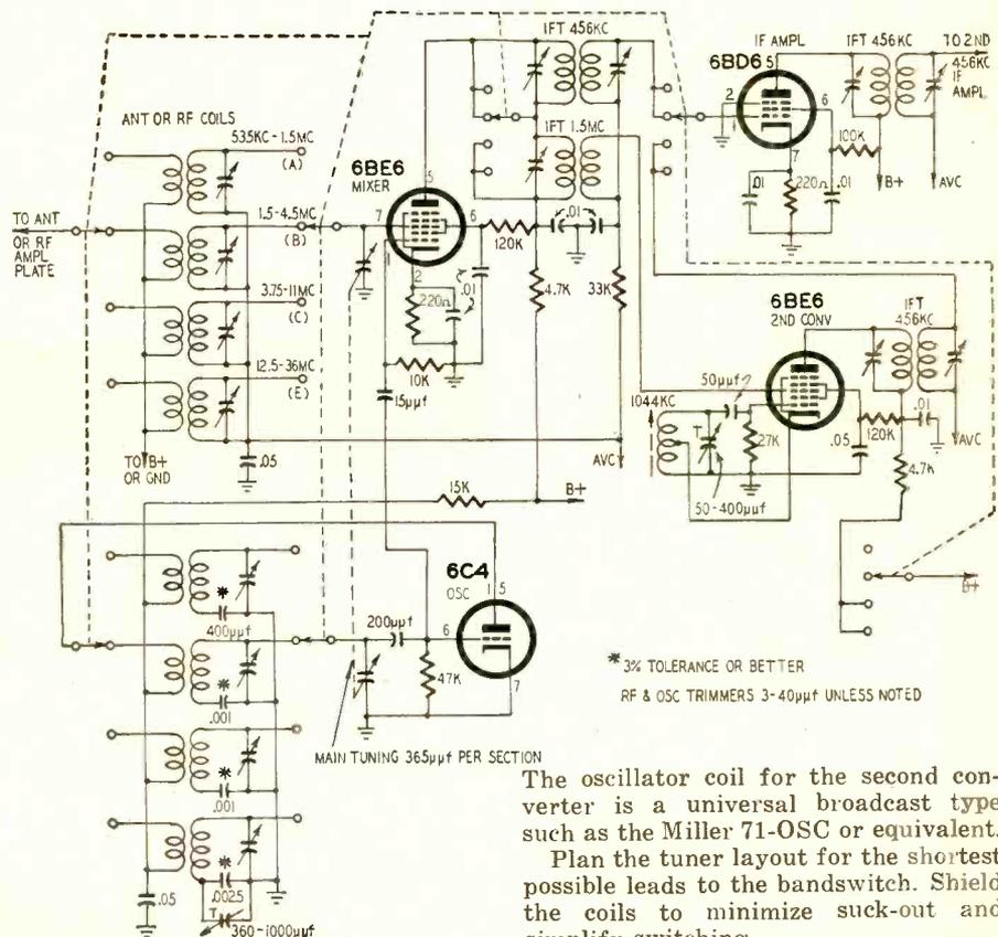
The oscillator coil for the second converter is a universal broadcast type such as the Miller 71-OSC or equivalent.
