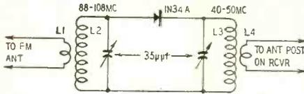
with this inexpensive tubeless converter (see diagram) connected between a good FM (88-108-mc) antenna and the antenna posts of their old FM receiver.
