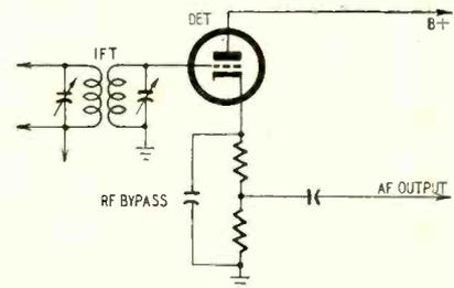
Fig. 3—Infinite-impedance detector.
