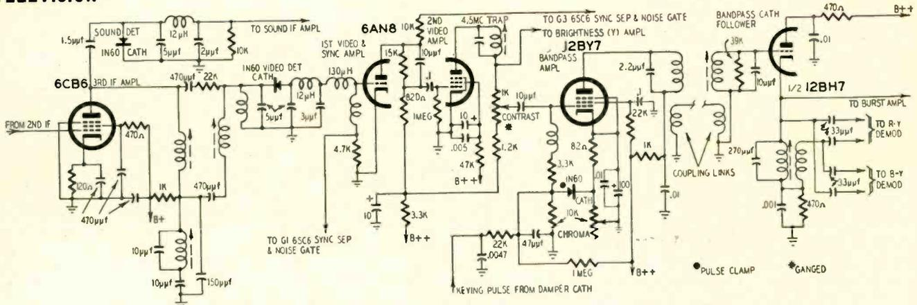
Fig. 2—The video circuits and sound detector following third i.f. amplifier.
