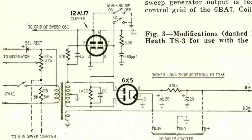
Fig. 3—Modifications (dashed lines) in Heath TS-3 for use with the adapter.
