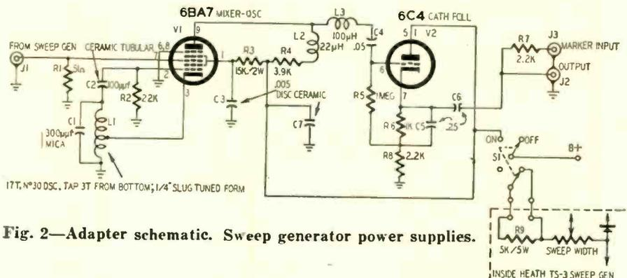
Fig. 2—Adapter schematic. Sweep generator power supplies.
