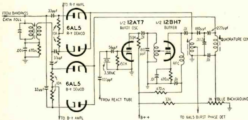
Fig. 4—Schematic of the demodulators, oscillator and quadrature circuits.
