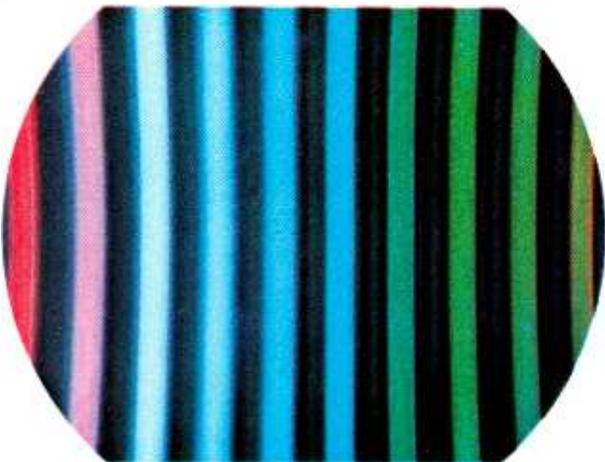
Fig. 5—An example of incorrect hue control adjustment.
