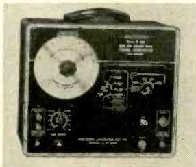
from 20 through 20,000 cycles in three bands. Square-wave signals at 50, 100, 250 and 500 kc. Output impedance on variable-frequency ranges: 0-2,000 ohms, 0-10 volts r.m.s. flat within ±1 db. Accuracy ±2% from 50 cycles to 200 kc, ±1 cycle from 20 to 50 cycles. Distortion: less than 1% from 20 cycles through 200 kc. Square-wave rise time at 20 kc: 0.5 microsecond.—Precision Apparatus Co., Inc., 92-97 Horace Harding Blvd., Elmhurst, L. I., N. Y.
