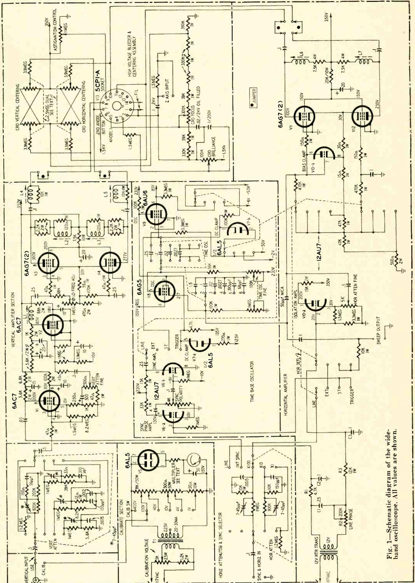
Fig. 1—Schematic diagram of the wide-band oscilloscope. All values are shown.
