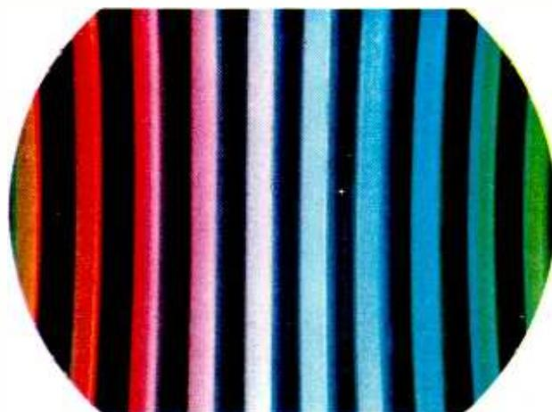
Fig. 1—Color bar pattern with fine tuning misadjusted.
