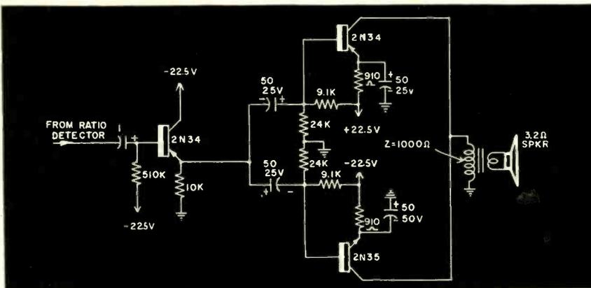
Fig. 5—The audio amplifier and complementary symmetry audio output stage.
