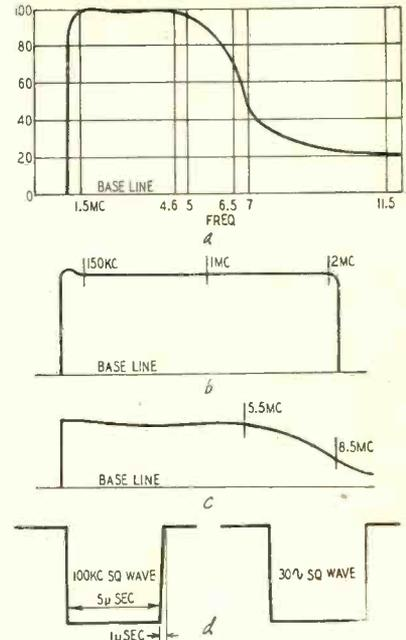
Fig. 3—Curve at *a* is desired response of the vertical amplifier measured at the deflection plates of the C-R tube. Sweep trace *b* shows low-frequency responses at the vertical plates of the 5CP1-A. Response at plate of compensated 6AC7 is shown at *c*. Square waves at *d*, like the trace at *b*, show low-frequency response at vertical plates of C-R tube. Patterns traced from RCA scope.
