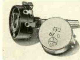
Terminals directly fastened to winding, insuring low contact resistance and improving end termination. Collector and terminal in one piece, eliminating rivets as mechanical fasteners and current conductors. Stop is integral with base instead of in the cover.—Clarostat Manufacturing Co. Inc., Dover, N. H.
