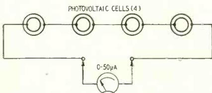
The instrument consists of four inexpensive photovoltaic cells and a 50- $\mu$ a d.c. meter or the basic range of a 20,000-ohms-per-volt voltmeter connected as shown in the diagram. The cells are mounted on a flat bakelite strip in a suitable housing that can be suspended against the screen by the meter leads. (For details on a simple mounting arrangement, see "Transistorized Commercial Killer" in the July, 1954, issue.—*Editor*)
