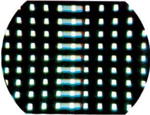
Fig. 3—Appearance of a properly converged dot pattern.
