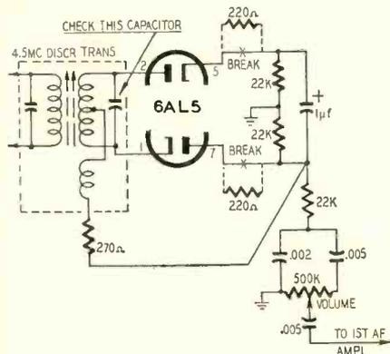
sound discriminator circuit. If careful lead dress does not reduce or remove it, check the capacitor across the sec-
