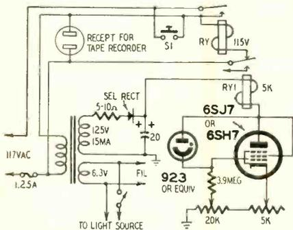
The control circuit obtains power from a half-wave type power transformer (a Stancor PS-8415) but can take its power—100–150 volts at about 10 ma—from any radio or amplifier operated with the recorder. The plate-circuit relay is a Potter & Brumfield LM-5 with a 5,000-ohm coil. A 923 phototube was used because it was readily available. Other types can be substituted. A miniature 3S4 or a 3Q5-GT can be substituted for the 6SJ7 or 6SH7 shown by changing the filament supply to 3 volts.
