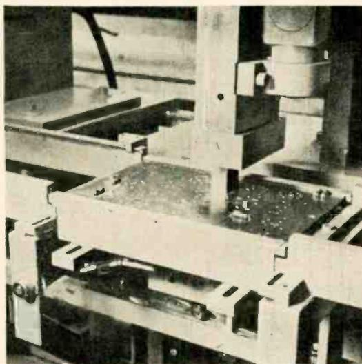
The machine at left inserts wire jumpers that connect the circuits on a printed-circuit board.
