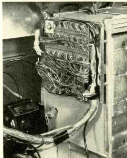
Fig. 2—Connection board on reed chamber.
