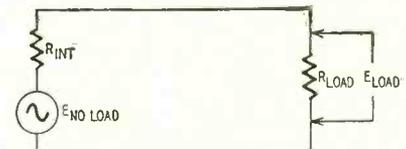
Fig. 1—Equivalent output circuit.
