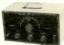
The Heathkit Audio Oscillator will produce both sine and square waves within the frequency range from 20 CPS to 20 KC in three ranges. Thermistor controlled linearity results in a variation of no more than ±1 db in a 10 volt (no load) variable output level. There will be less than .6% distortion from 100 CPS throughout the audible range. Low impedance 600 ohm output. Precision 1% resistors, used in the range multiplier circuits to provide accurate calibration.
