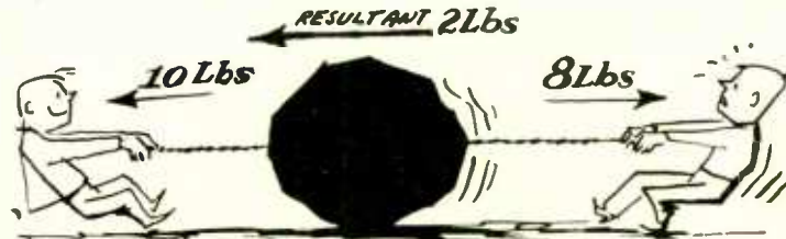
Fig. 2—Two forces acting on one object. The net acting force is the difference.
