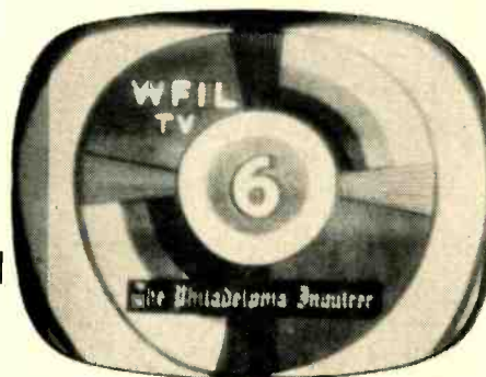
Fig. 1—Picture due to low line supply voltage.
