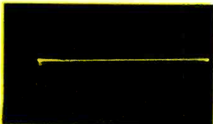
Fig. 1—Signal tracing with crystal probe shows dead stage as a horizontal line.
