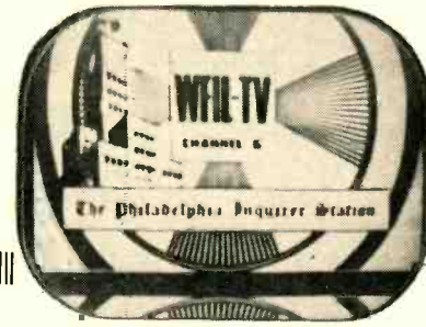
Fig. 4—Rolling the picture slowly as a means of checking vertical linearity.
