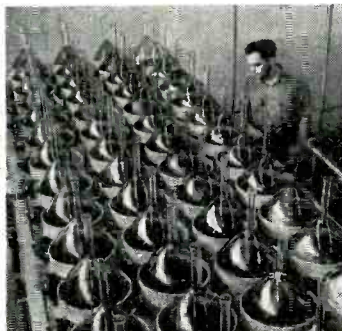
The completed electron guns shown in the photo above are being carefully aligned for proper operation. The picture tube bulbs at right are thoroughly washed to prevent contamination of fluorescent material.
