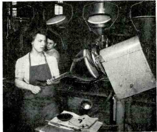
The operator above is putting a coat of conductive material on the inside of a large glass picture tube.
