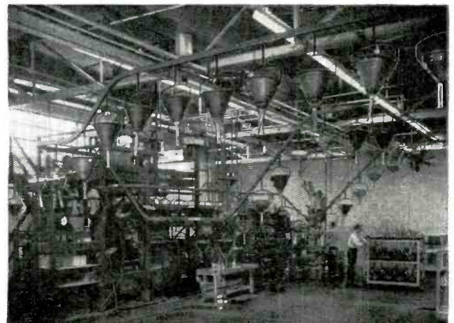
Overhead conveyers and other automatic equipment provide a continuous efficient movement of tubes during production.
