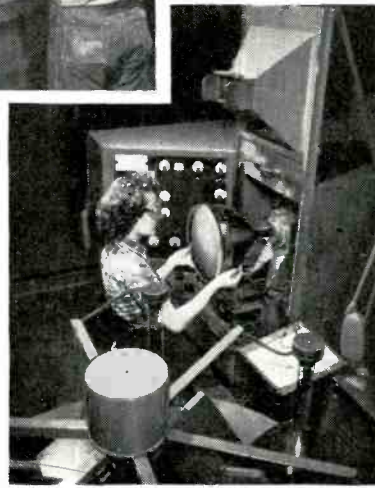
After coating and screening, the bulbs go through a high-temperature oven to drive out all organic matter. The operator above takes the bulbs from the conveyer as they emerge from the oven and puts them on the overhead conveyer which takes them on to the next step.
