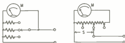
Fig. 1, left—A shunt for each range. Fig. 2, right—The Ayrton or ring shunt.
