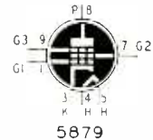
Base diagrams of some of the new tubes.
