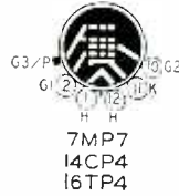
Base diagrams of some of the new tubes.
