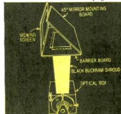
Fig. 3—The optical system is shielded from stray light and dust by a shroud.
