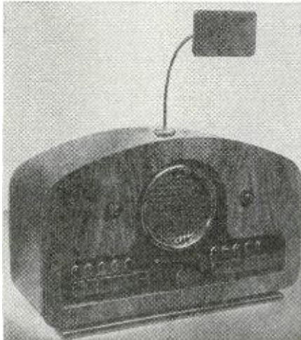
Body capacitance switches the intercom.
