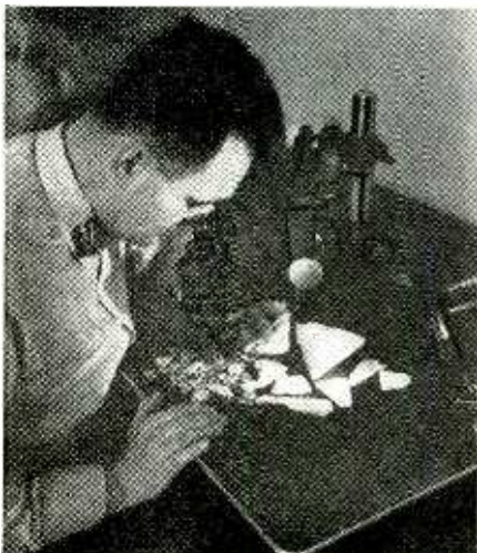
Flakes of new mica are examined by microscope for possible structural defects.
