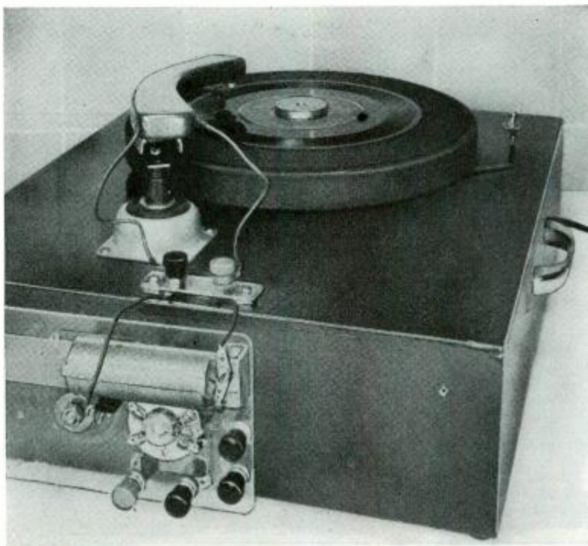
The oscillator needed for the FM pickup is fastened to the rear of the cabinet.
