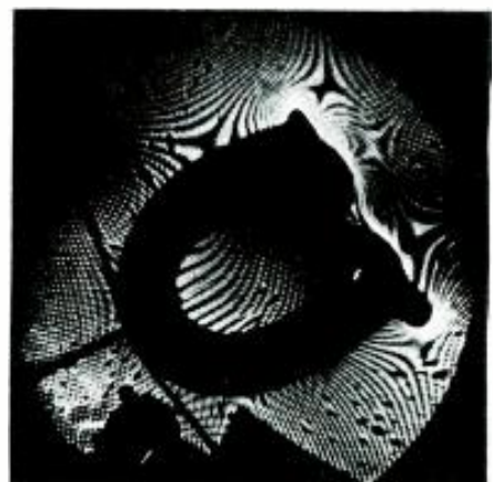
Fig. 4—Pattern of a horseshoe magnet.
