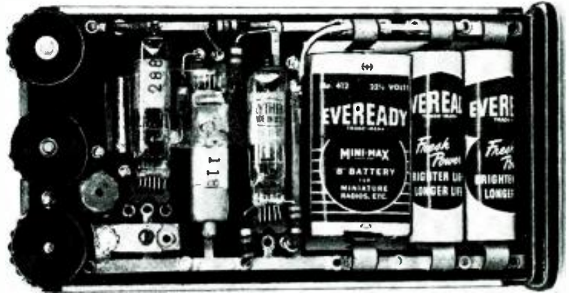
This side of chassis shows how the tube "pins" are bent and pushed in sockets.
