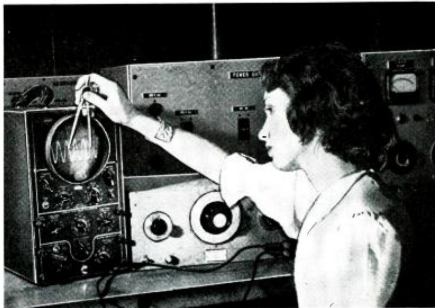
Machinist's dividers are used to compare shutter opening with audio sine waves.
