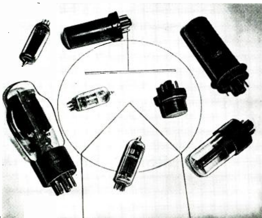
These are a few of the common diodes—all sizes and ratings are manufactured.
