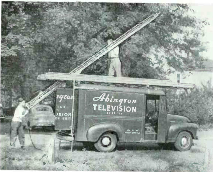
Mobile research truck houses 68-foot collapsible antenna tower, TV set, and test gear.
