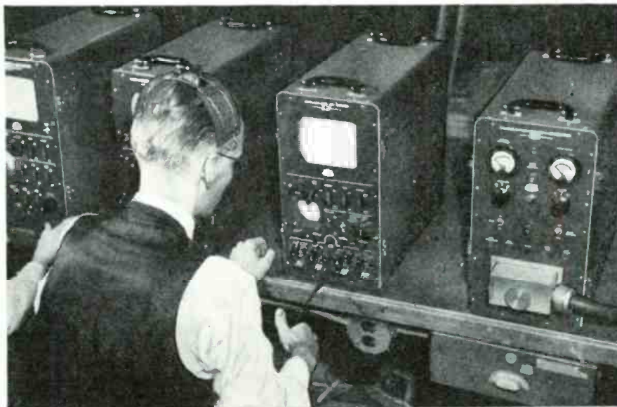
Fig. 3—All pix signals go to mixer (second from right). This is a portable control setup. Courtesy Allen S. Du Mont Laboratories, Inc.
