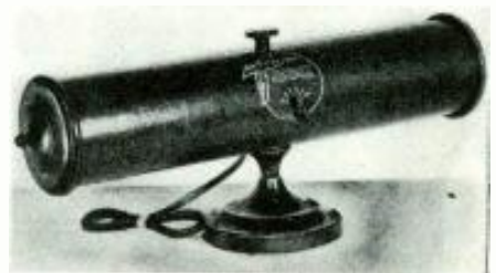
Fig. 5-b—Cylindrical antenna with tuning.
