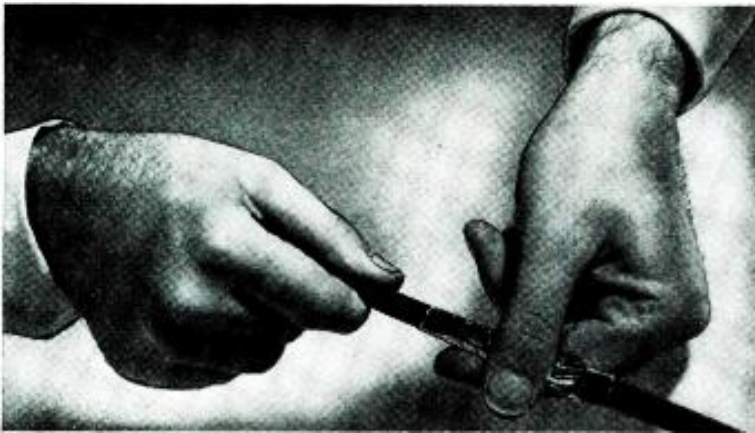
This photo shows the strip of tinfoil wrapped around the line and held in place with a clip.
