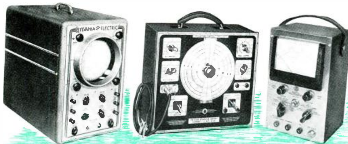
A standard signal generator with 400-cycle modulation and an output meter are necessities.
