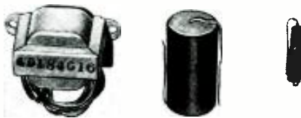
Chief actors—inductor, capacitor, resistor.
