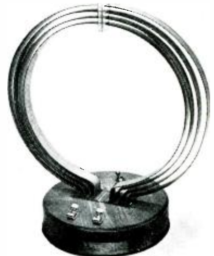
An early model of the antenna had fixed loops.
