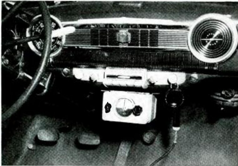
T-17 microphone hangs beside the converter. Both are handy to the driver.
