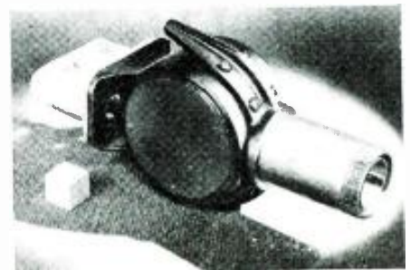
Fig. 8—A 20-kw magnetron, the W.E. 728-AJ, connected in parallel. These and other special types are either outmoded or have little general application and are interesting only from a purely academic viewpoint.
