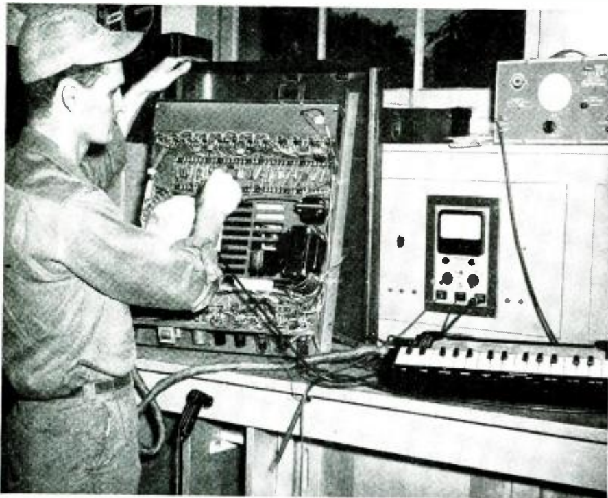
The author has taken the "works" out of the tone cabinet for service. Keyboard is at right.
