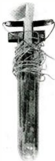
This test tube was cracked when Carnauba wax was cooled in intense electric field.
